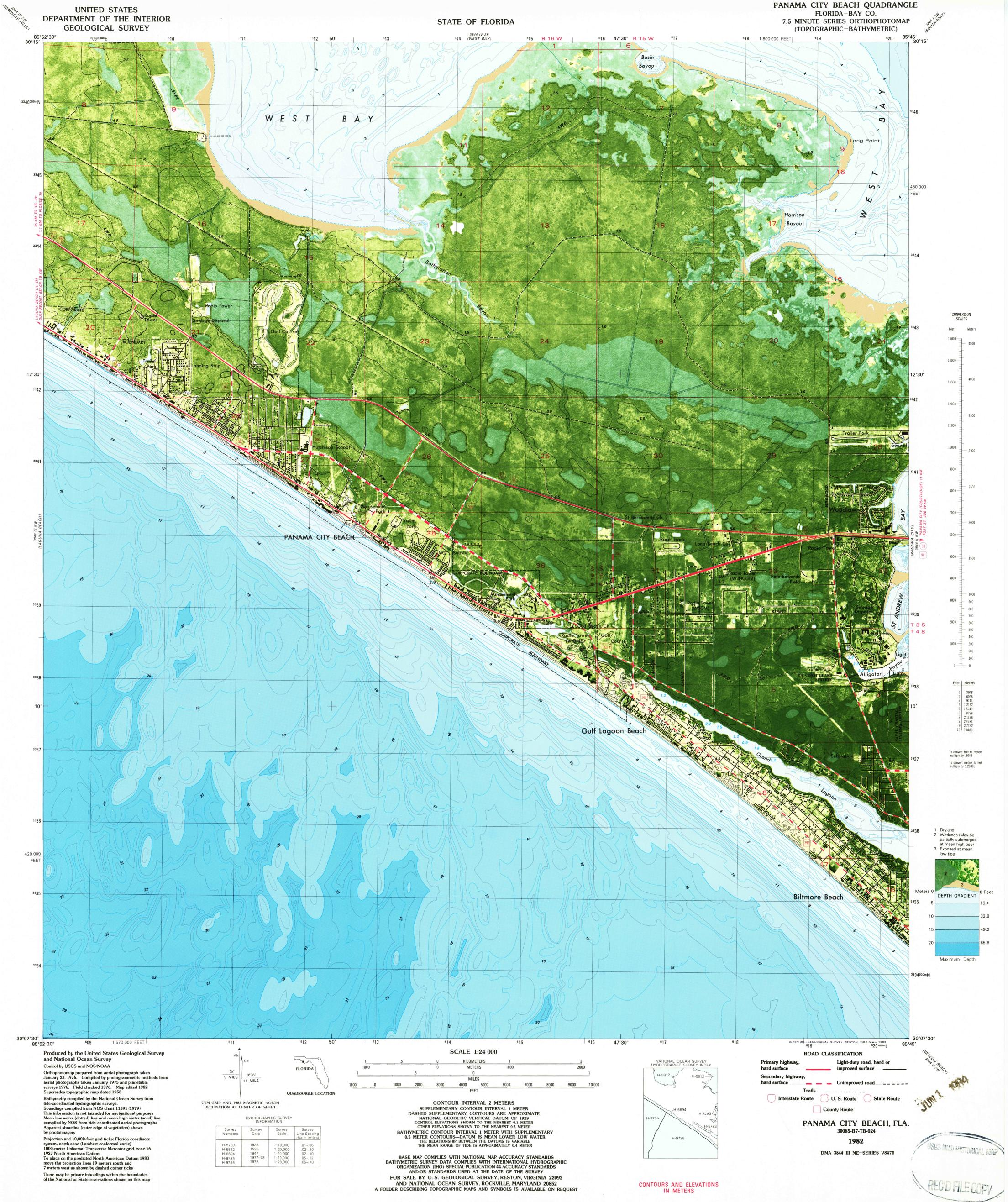
Projection and 10,000-foot grid ticks: Florida coordinate system, north zone (Lambert conformal conic) 1000-meter Universal Transverse Mercator grid, zone 16 1927 North American Datum To place on the predicted North American Datum 1983 move the projection lines 19 meters south and 7 meters west as shown by dashed corner ticks
