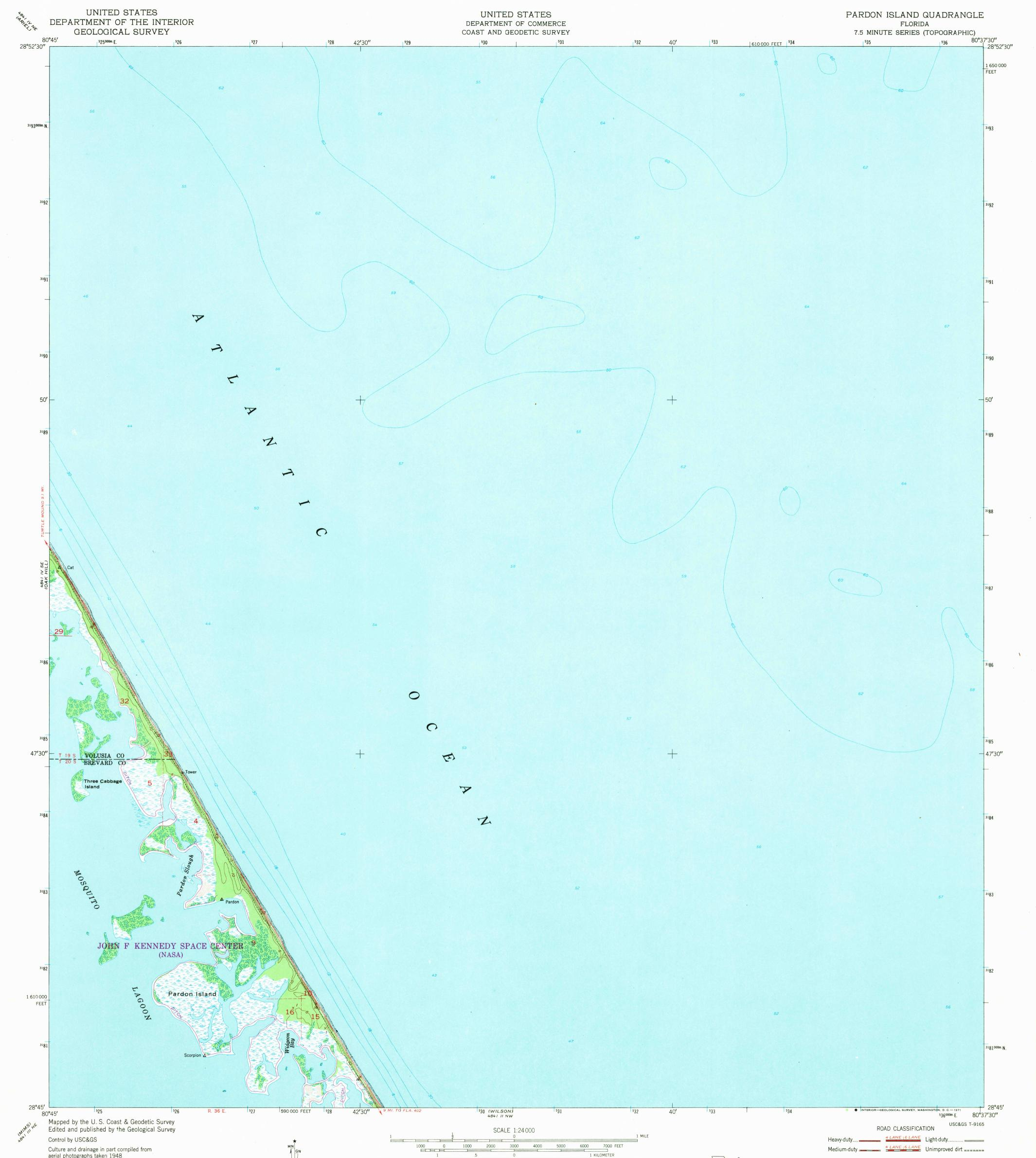
aerial photographs taken 1948 Topography by plane-table methods 1949. Field check 1949 Hydrography compiled from charts surveyed 1948 Polyconic projection 1927 North American Datum 10,000 foot grid based on Florida coordinate system, east zone Dashed land lines indicate approximate location 1000-meter Universal Transverse Mercator grid ticks, zone 17, shown in blue
