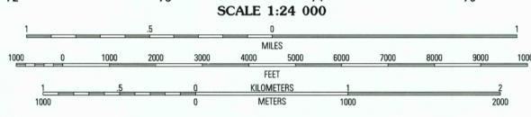
CONTOUR INTERVAL 5 FEET NATIONAL GEODETIC VERTICAL DATUM OF 1929 TO CONVERT FROM FEET TO METERS, MULTIPLY BY 0.3048
