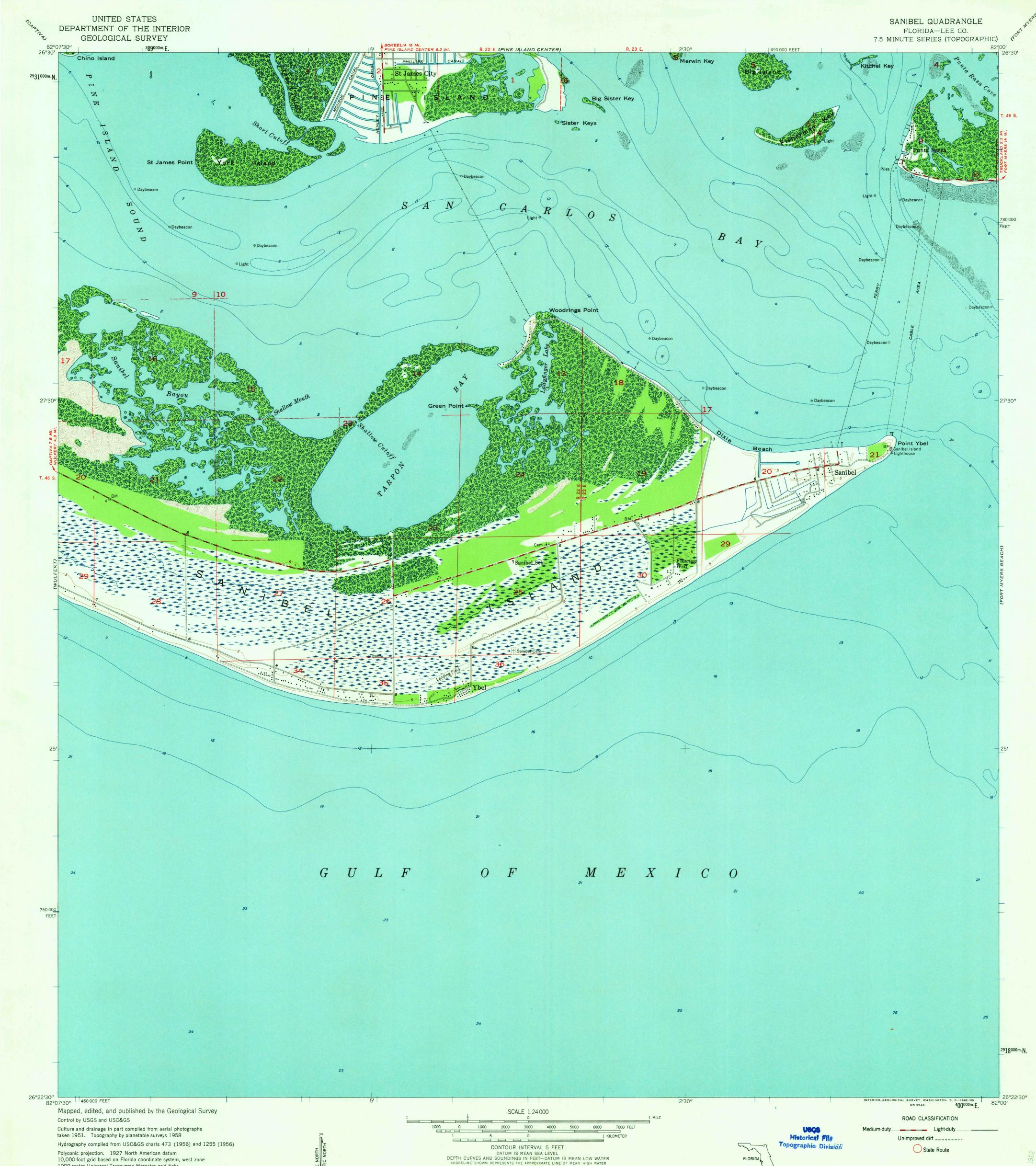
Polyconic projection. 1927 North American datum 10,000-foot grid based on Florida coordinate system, west zone 1000-meter Universal Transverse Mercator grid ticks, zone 17, shown in blue
