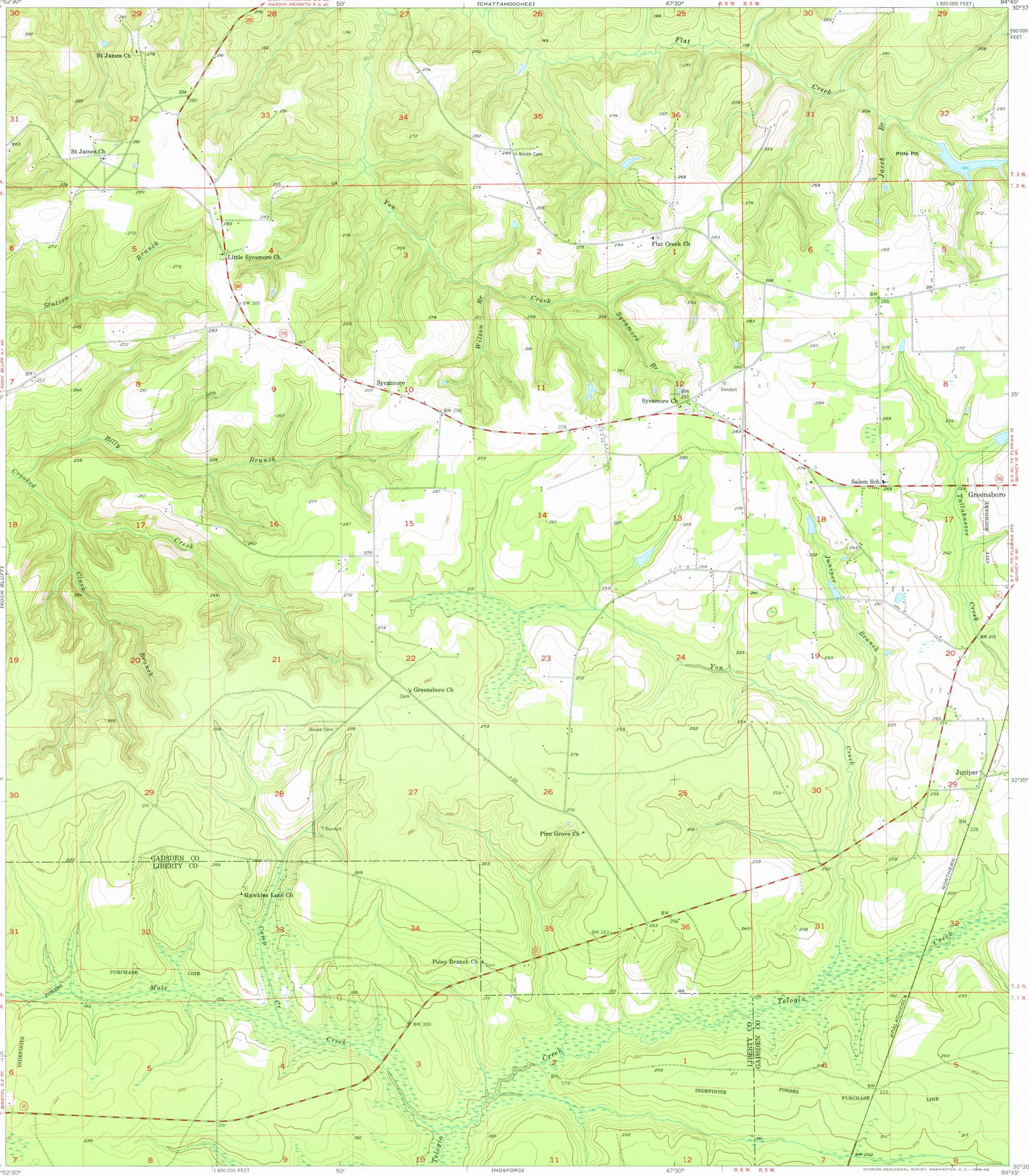
Mapped, edited, and published by the Geological Survey Control by USGS and USC&GS Culture and drainage in part compiled from aerial photographs taken 1947. Topography by planetable surveys 1954-1955 Polyconic projection. 1927 North American datum 10,000-foot grid based on Florida coordinate system, north zone Dotted land lines were established by private subdivision of the Forbes Purchase
