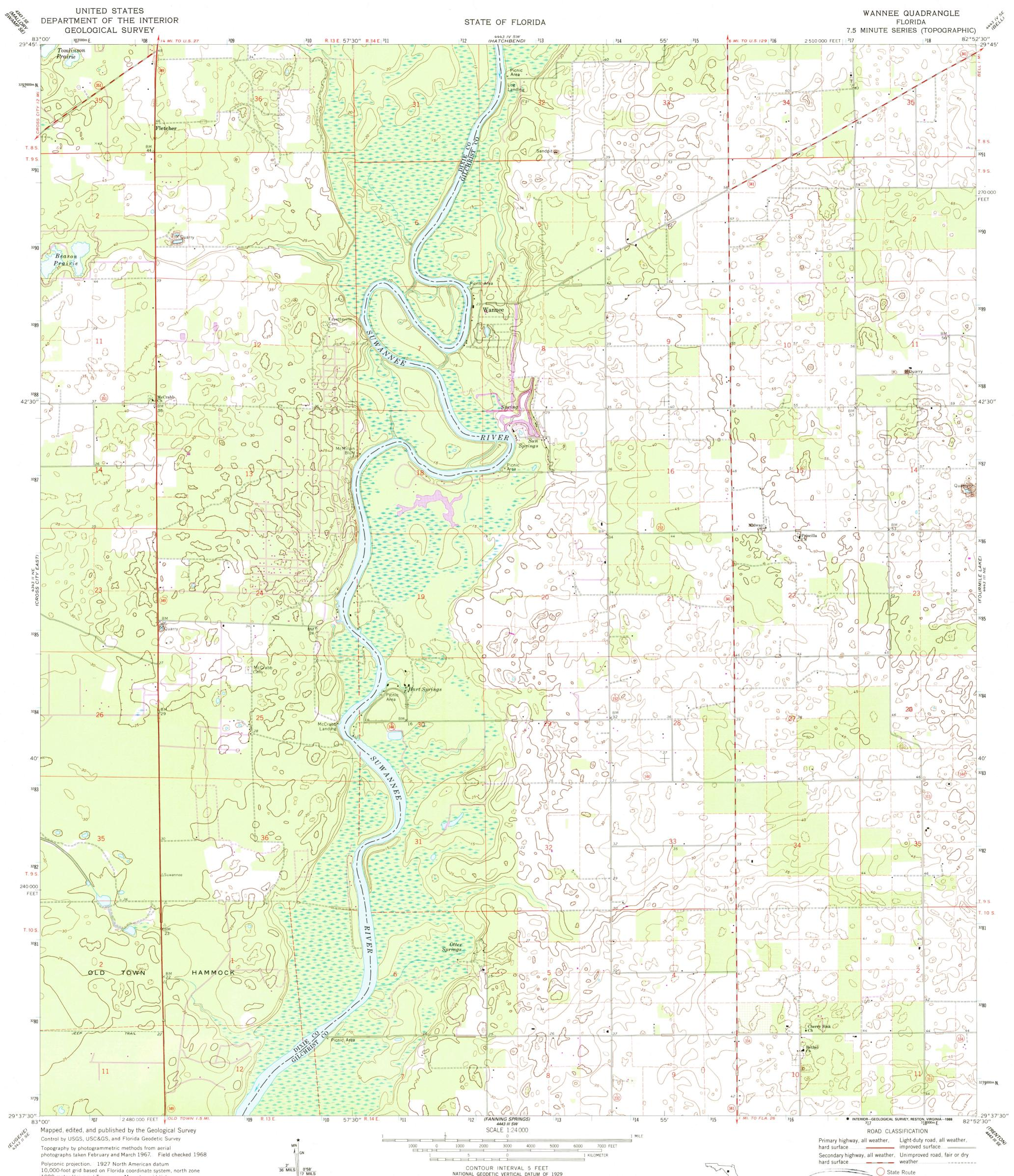
10,000-foot grid based on Florida coordinate system, north zone 1000-meter Universal Transverse Mercator grid ticks, zone 17, shown in blue
