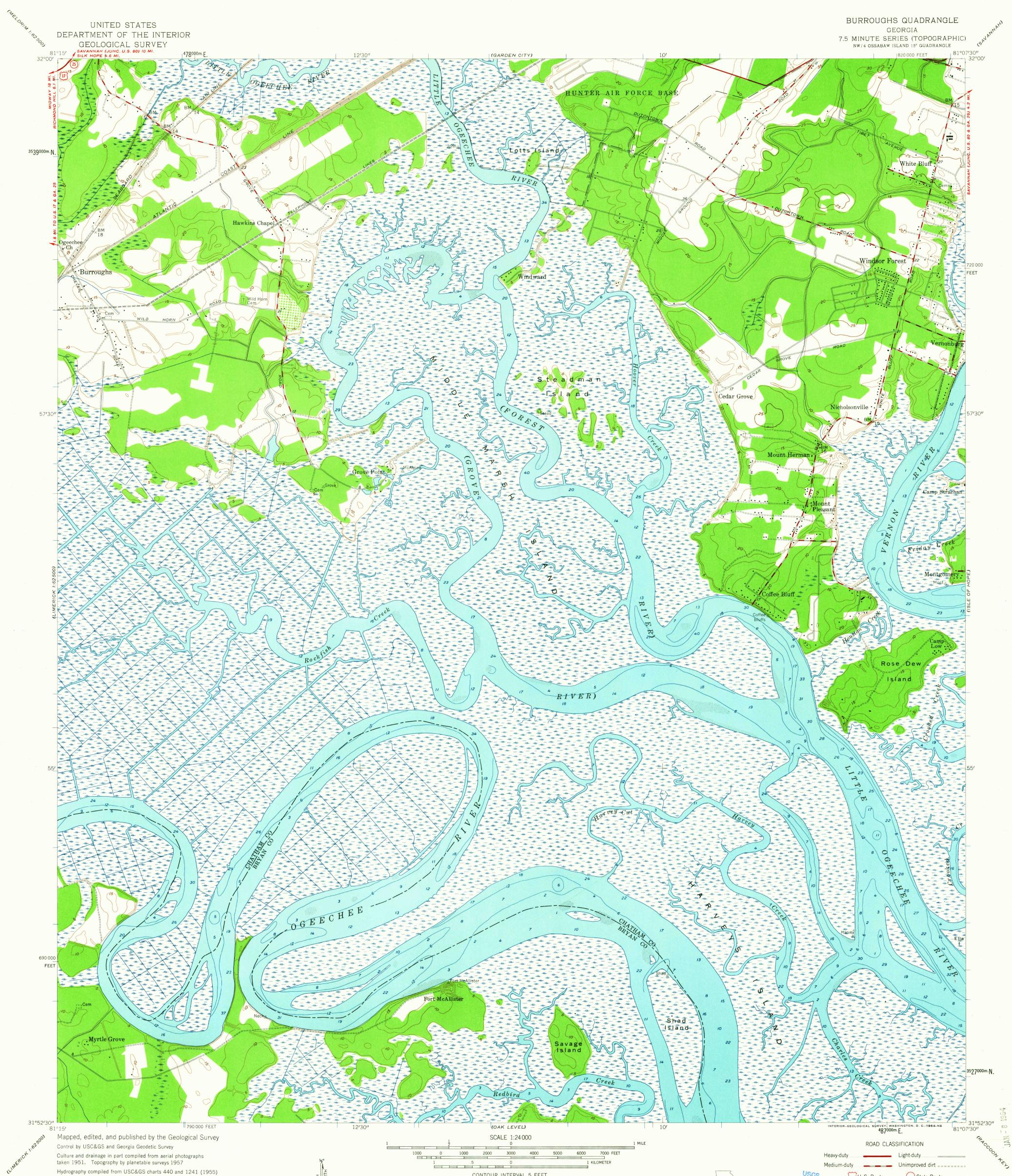
taken 1951. Topography by planetable surveys 1957 Hydrography compiled from USC&GS charts 440 and 1241 (1955) Polyconic projection. 1927 North American datum 10,000-foot grid based on Georgia coordinate system, east zone 1000-meter Universal Transverse Mercator grid ticks,
