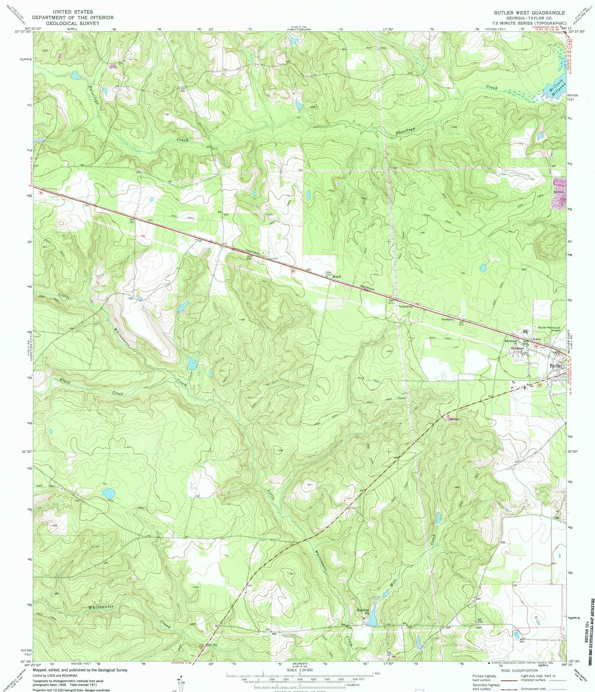
Projection and 10,000-foot grid ticks: Georgia coordinate system, west zone (transverse Mercator) 1000-meter Universal Transverse Mercator grid ticks, zone 16, shown in blue 1927 North American Datum To place on the predicted North American Datum 1983 move the projection lines 13 meters south and 9 meters west as shown by dashed corner ticks
