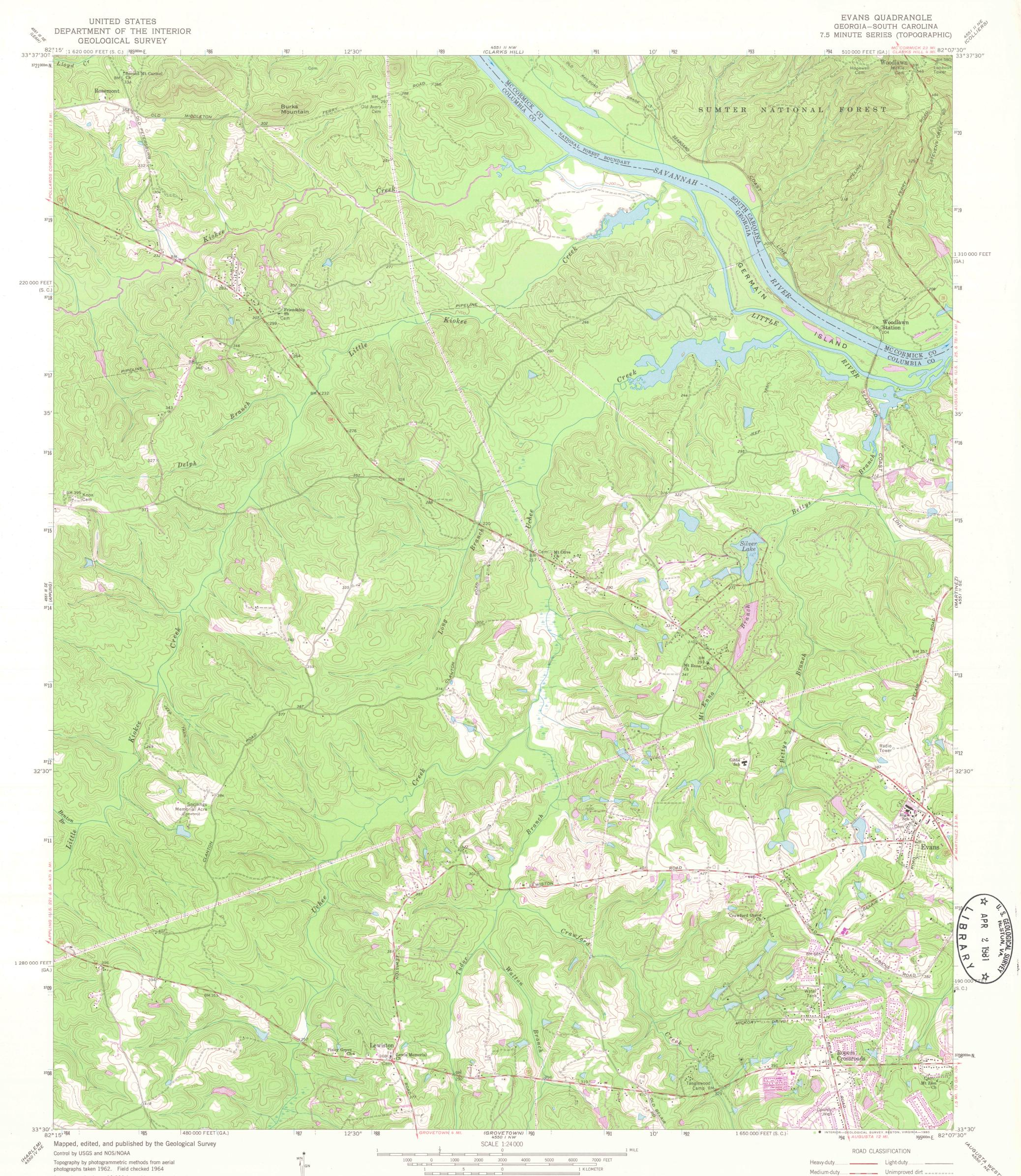
Polyconic projection. 10,000-foot grids based on Georgia coordinate system, east zone, and South Carolina coordinate system, north zone 1000-meter Universal Transverse Mercator grid ticks, zone 17, shown in blue. 1927 North American Datum To place on the predicted North American Datum 1983 move the projection lines 12 meters south and 14 meters west as shown by dashed corner ticks
