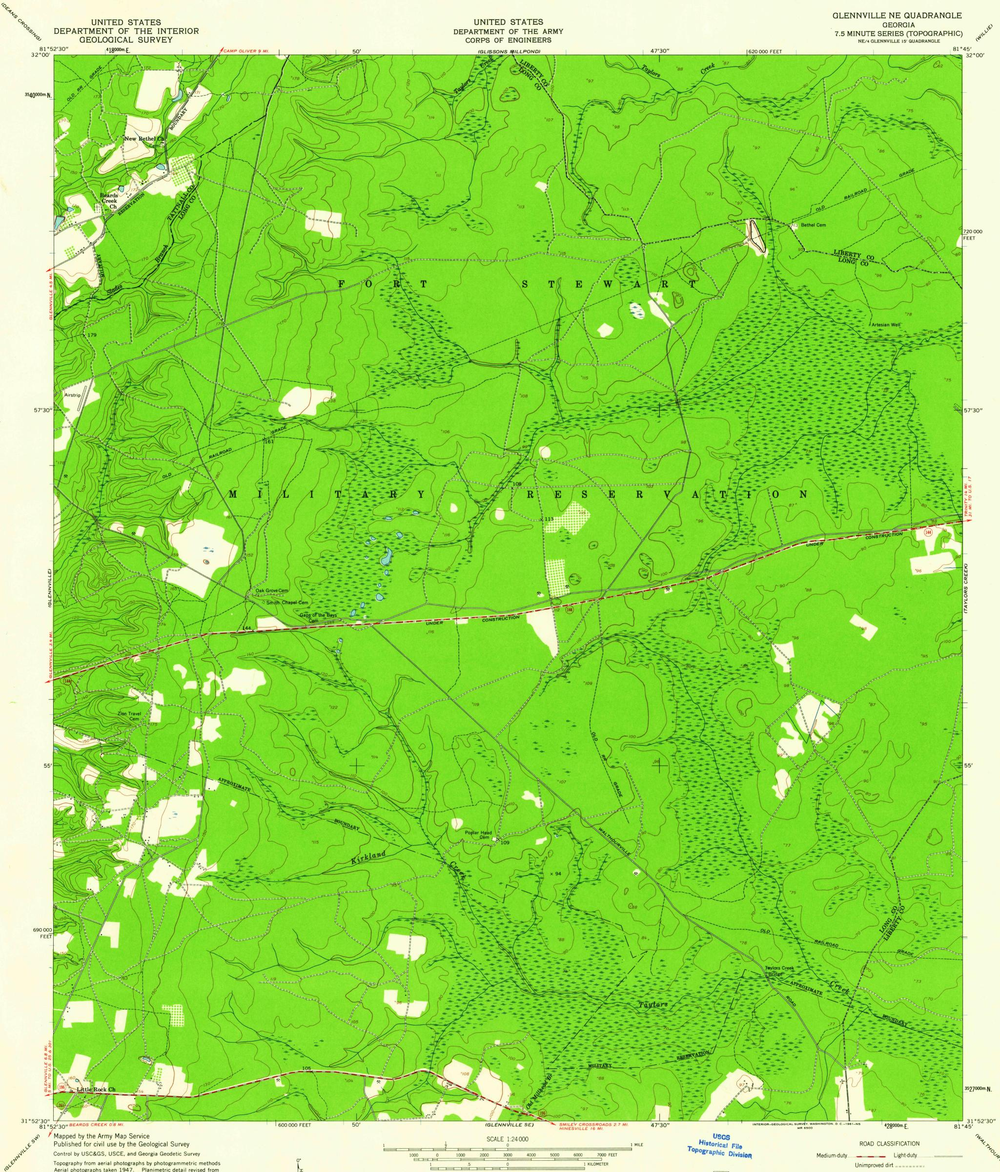
Topography from aerial photographs by photogrammetric methods Aerial photographs taken 1947. Planimetric detail revised from aerial photographs taken 1957. Field check 1958 Polyconic projection. 1927 North American datum 10,000-foot grid based on Georgia coordinate system, east zone 1000-meter Universal Transverse Mercator grid ticks, zone 17, shown in blue
