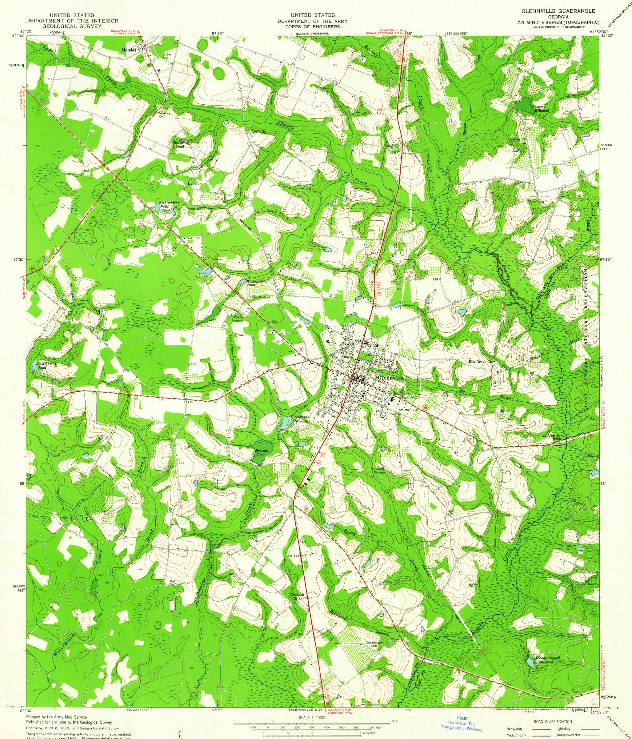
Topography from aerial photographs by photogrammetric methods Aerial photographs taken 1947. Planimetric detail revised from aerial photographs taken 1957. Field check 1958
