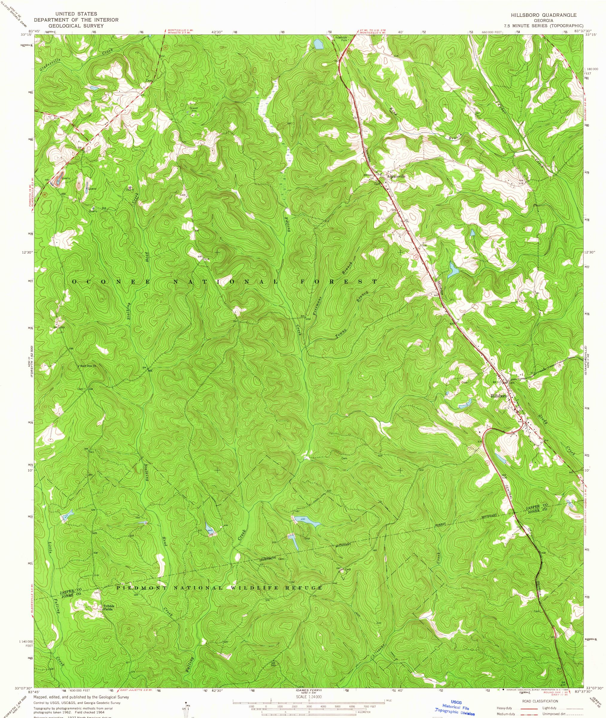
Polyconic projection. 1927 North American datum 10,000-foot grid based on Georgia coordinate system, west zone 1000-meter Universal Transverse Mercator grid ticks, zone 17, shown in blue
