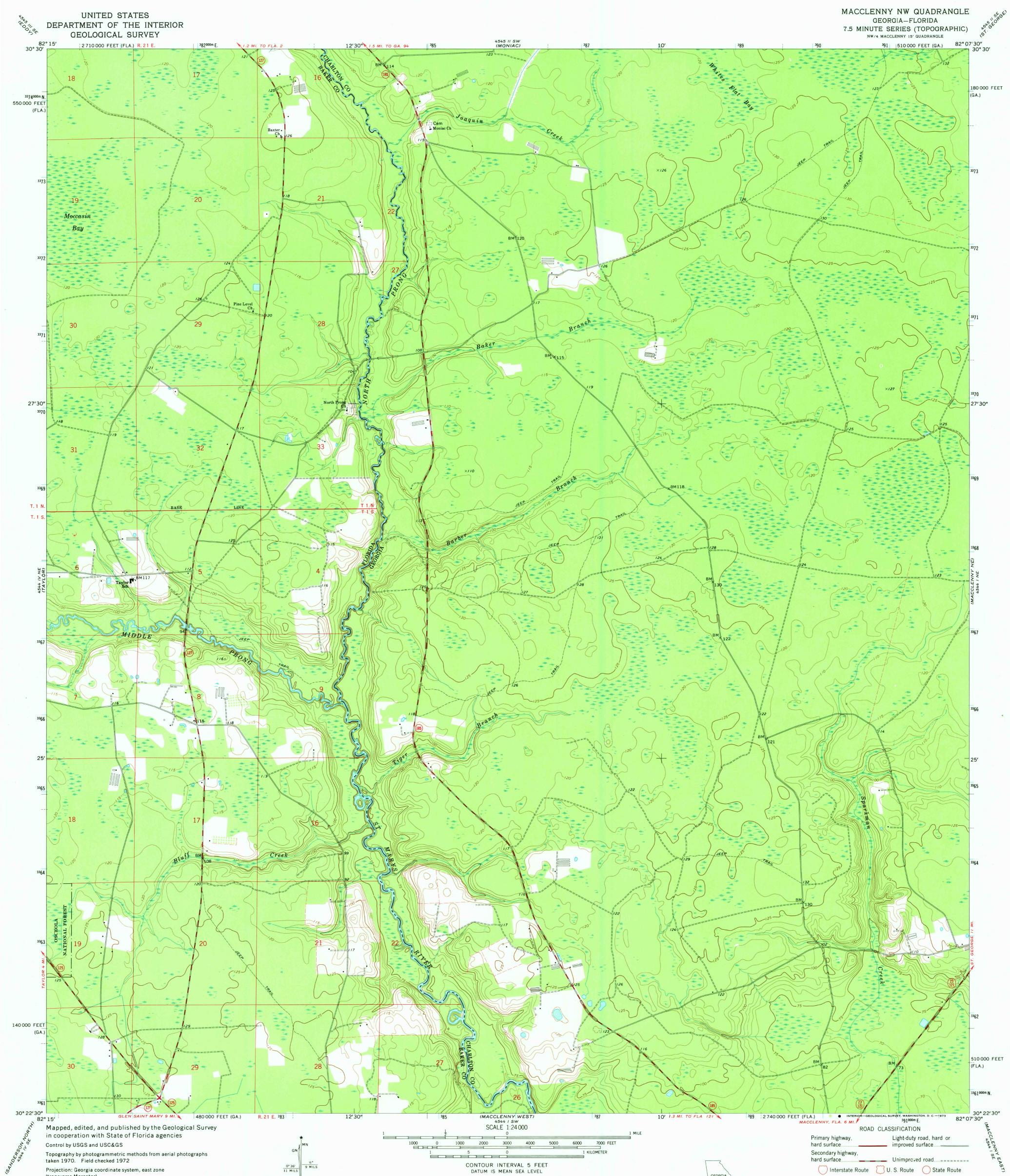
Projection: Georgia coordinate system, east zone (transverse Mercator) 10,000-foot grid ticks based on Georgia coordinate system, east zone and Florida coordinate system, north zone 1000-meter Universal Transverse Mercator grid ticks, zone 17, shown in blue. 1927 North American datum
