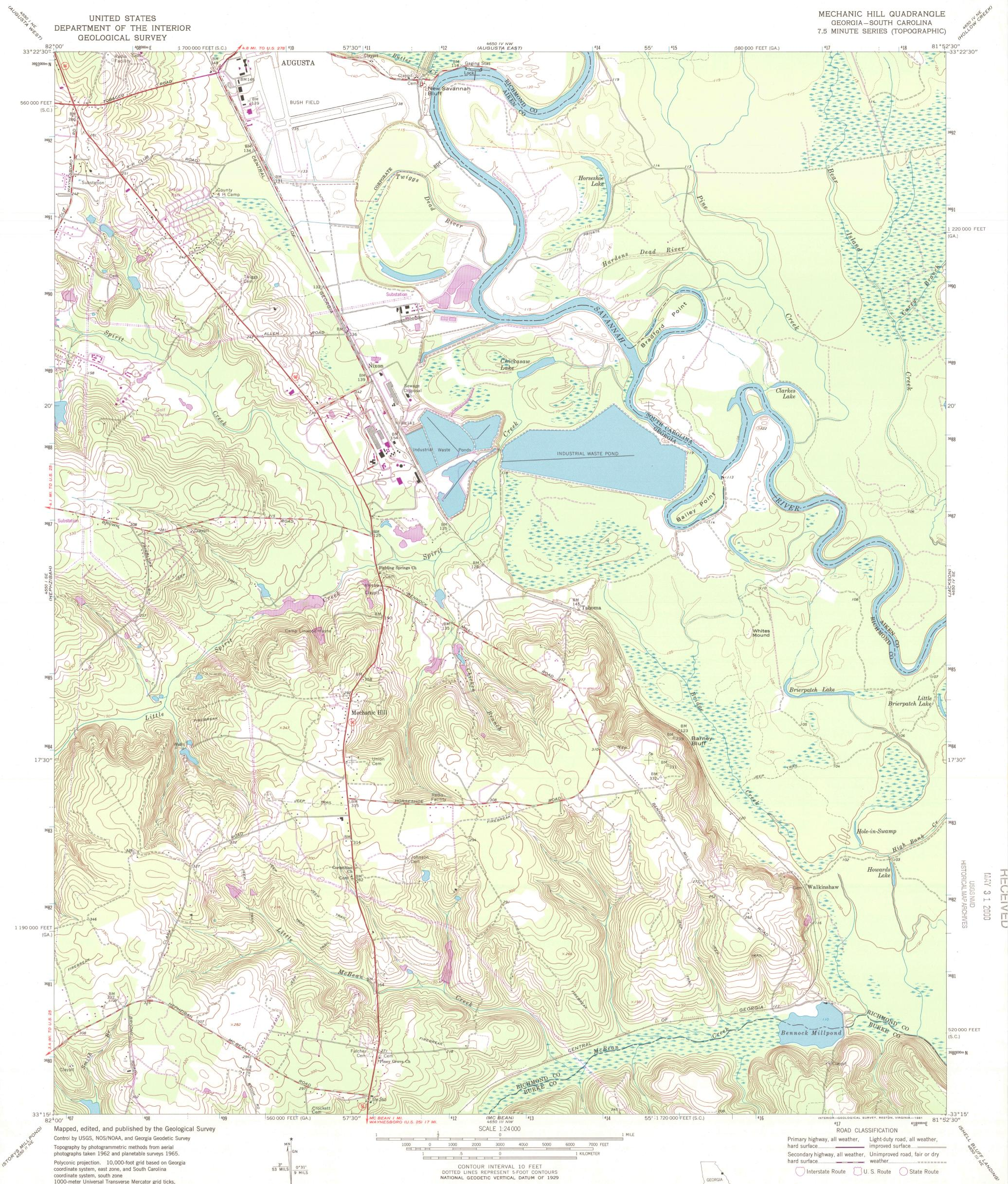
Polyconic projection. 10,000-foot grid based on Georgia coordinate system, east zone, and South Carolina coordinate system, south zone 1000-meter Universal Transverse Mercator grid ticks, zone 17, shown in blue. 1927 North American Datum To place on the predicted North American Datum 1983 move the projection lines 13 meters south and 15 meters west as shown by dashed corner ticks
