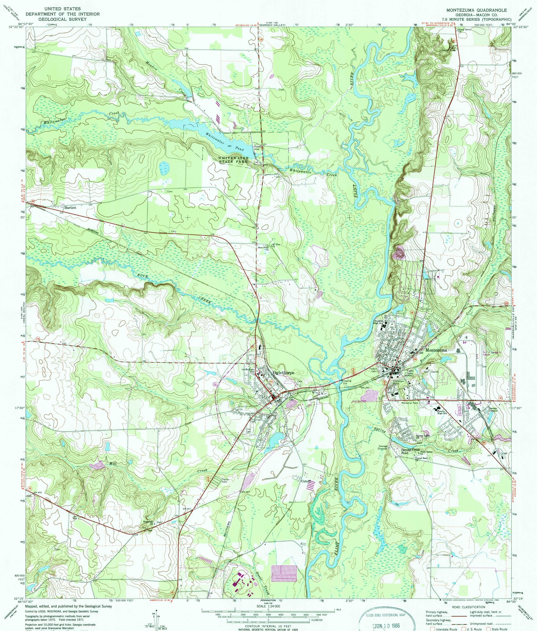
Projection and 10,000-foot grid ticks: Georgia coordinate system, west zone (transverse Mercator) 1000-meter Universal Transverse Mercator grid ticks, zone 16, shown in blue 1927 North American Datum To place on the predicted North American Datum 1983, move the projection lines 14 meters south and 9 meters west as shown by dashed corner ticks
