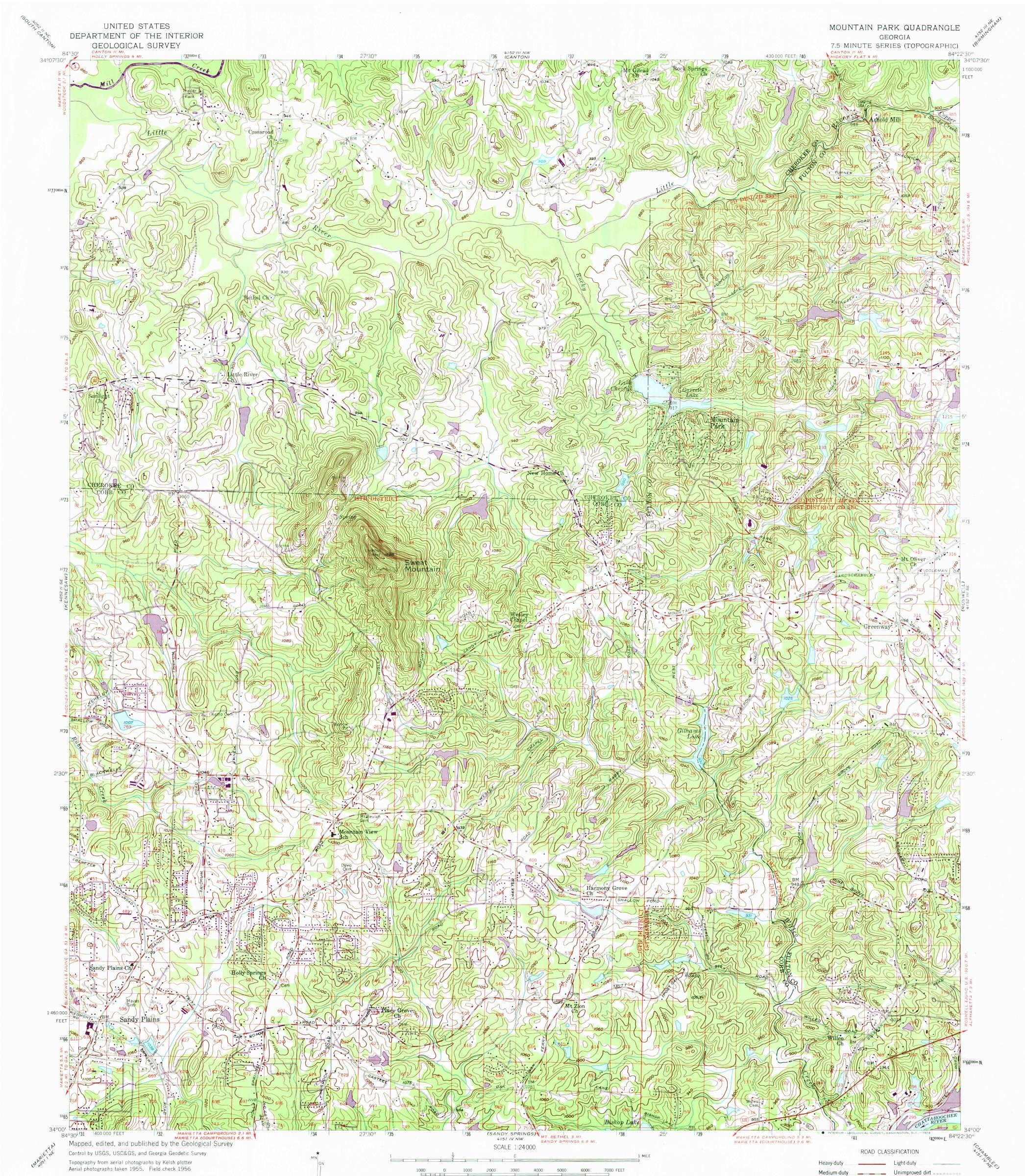
Polyconic projection. 1927 North American datum 10,000-foot grid based on Georgia coordinate system, west zone 1000-meter Universal Transverse Mercator grid ticks, zone 16, shown in blue
