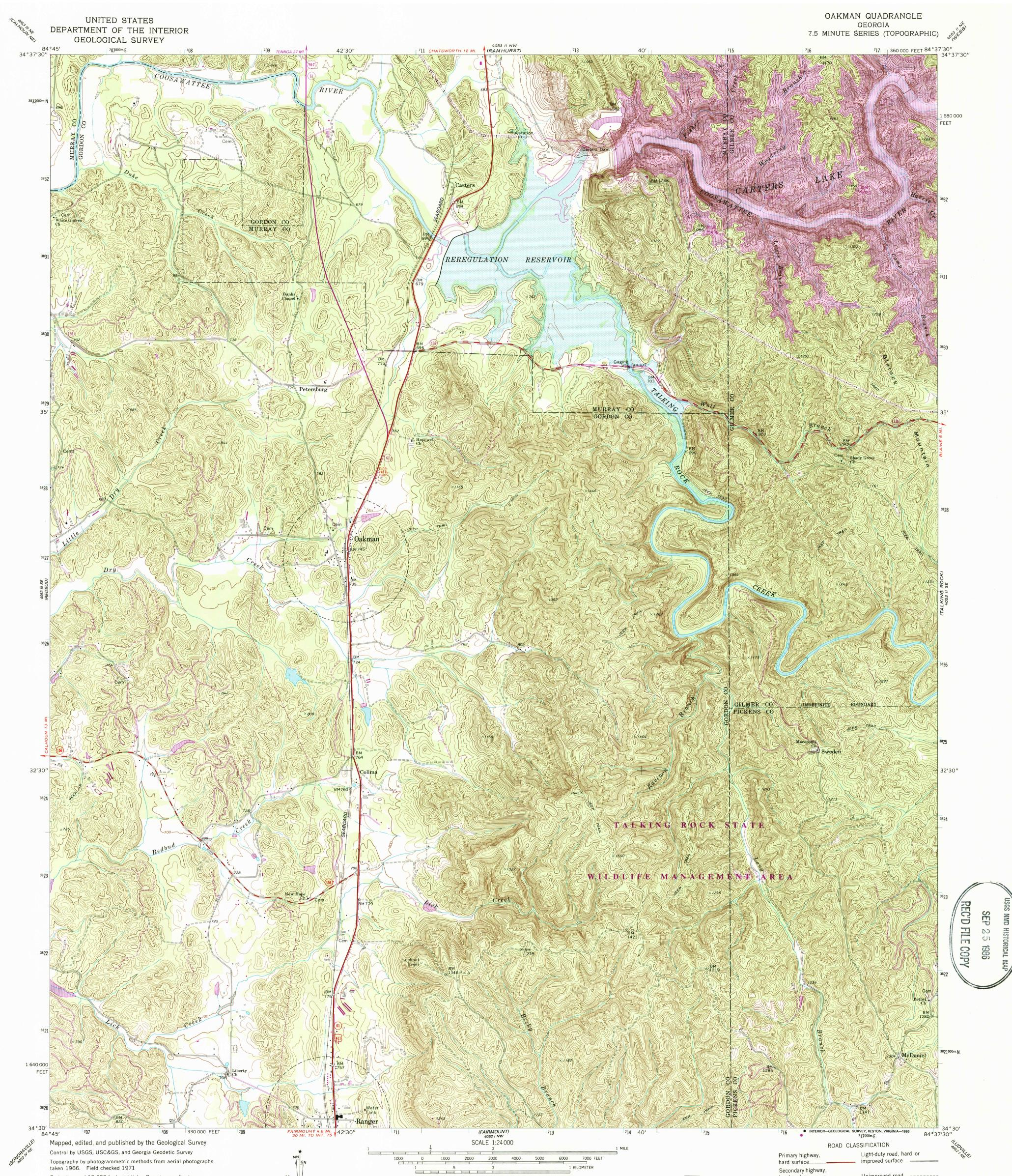
Projection and 10,000-foot grid ticks: Georgia coordinate system, west zone (transverse Mercator) 1000-meter Universal Transverse Mercator grid ticks, zone 16, shown in blue. 1927 North American datum To place on the predicted North American Datum 1983, move the projection lines 8 meters south and 6 meters west as shown by dashed corner ticks
