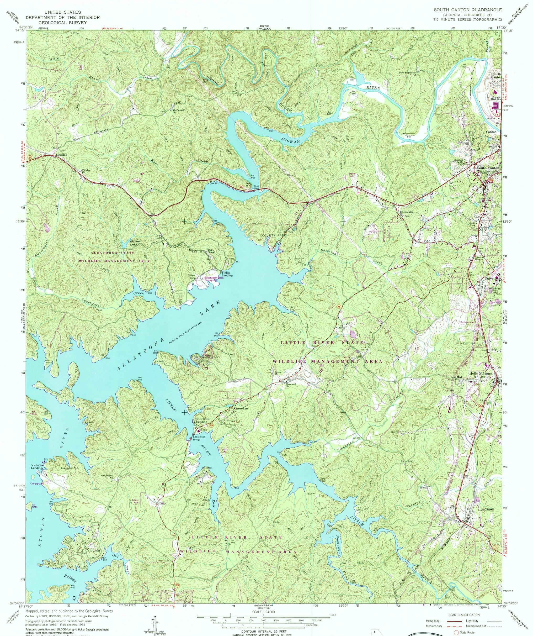
system, west zone (transverse Mercator) 1000-meter Universal Transverse Mercator grid ticks, zone 16, shown in blue. 1927 North American Datum To place on the predicted North American Datum 1983, move the projection lines 9 meters south and 7 meters west as shown by dashed corner ticks
