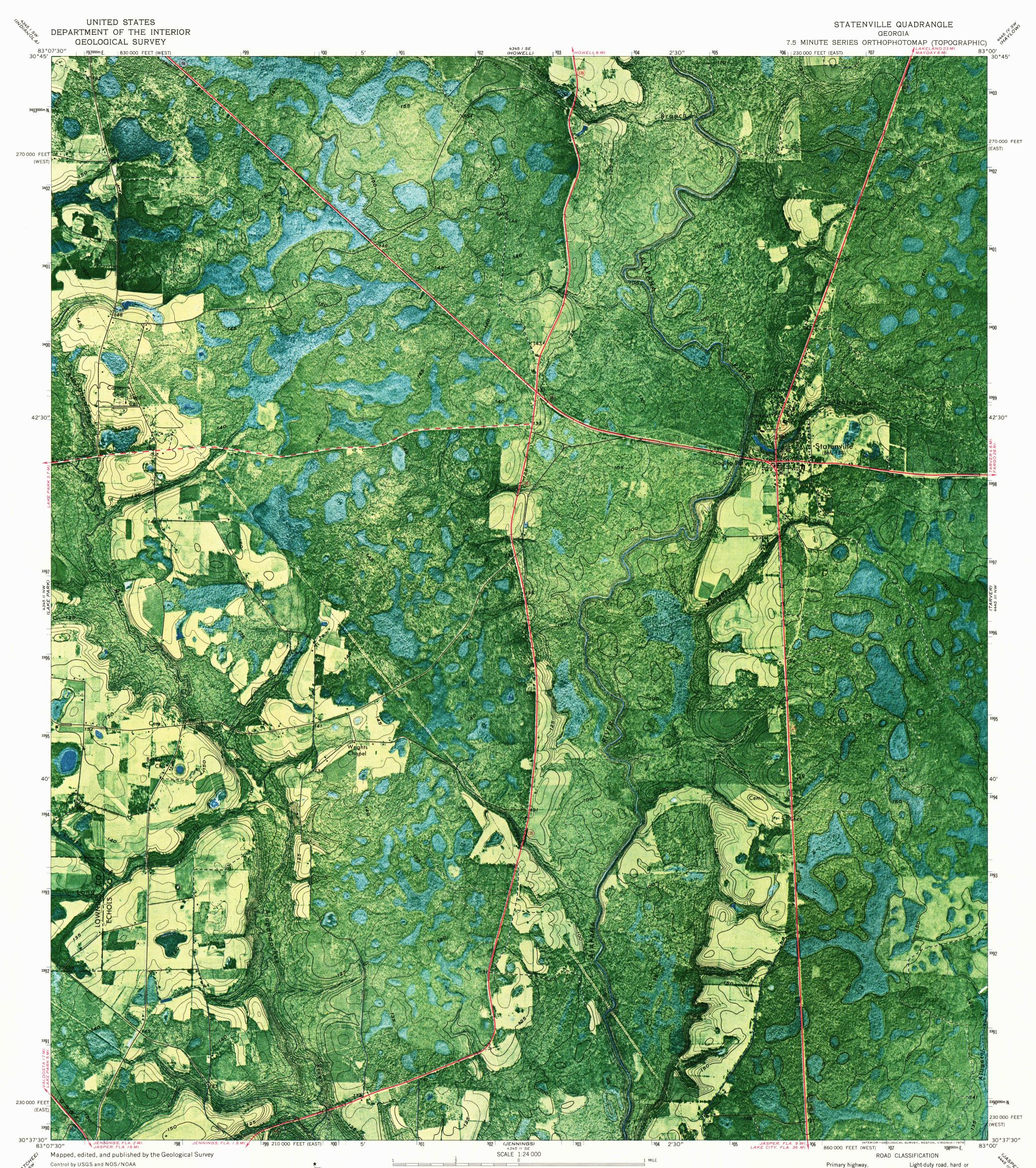
Orthophotomap prepared from aerial photographs taken January 1970 Topography by photogrammetric methods. Field checked 1971
