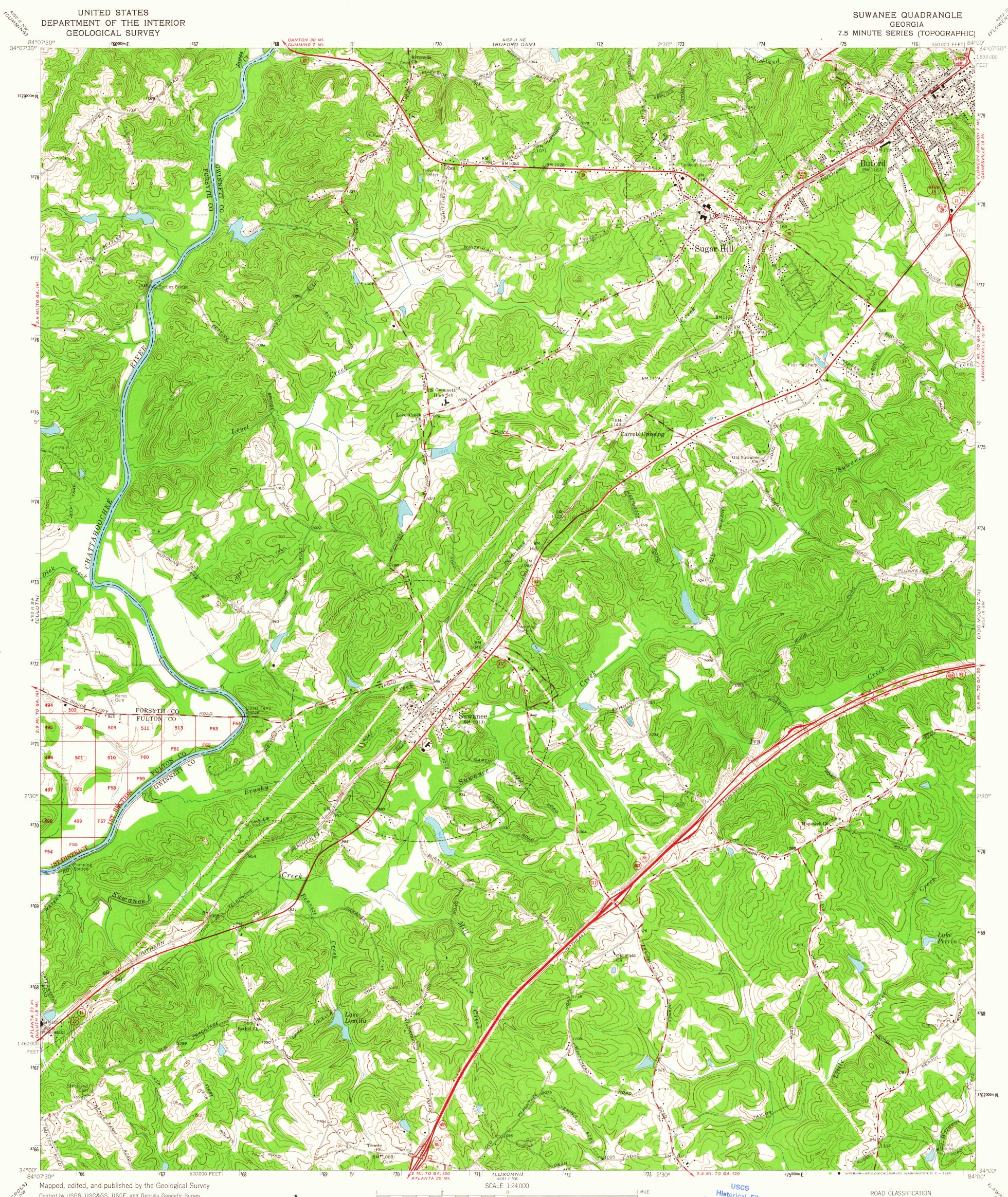
Control by USGS, USC&GS, USCE, and Georgia Geodetic Survey Topography by photogrammetric methods from aerial photographs taken 1956 and 1963. Field checked 1964 Polyconic projection. 1927 North American datum
