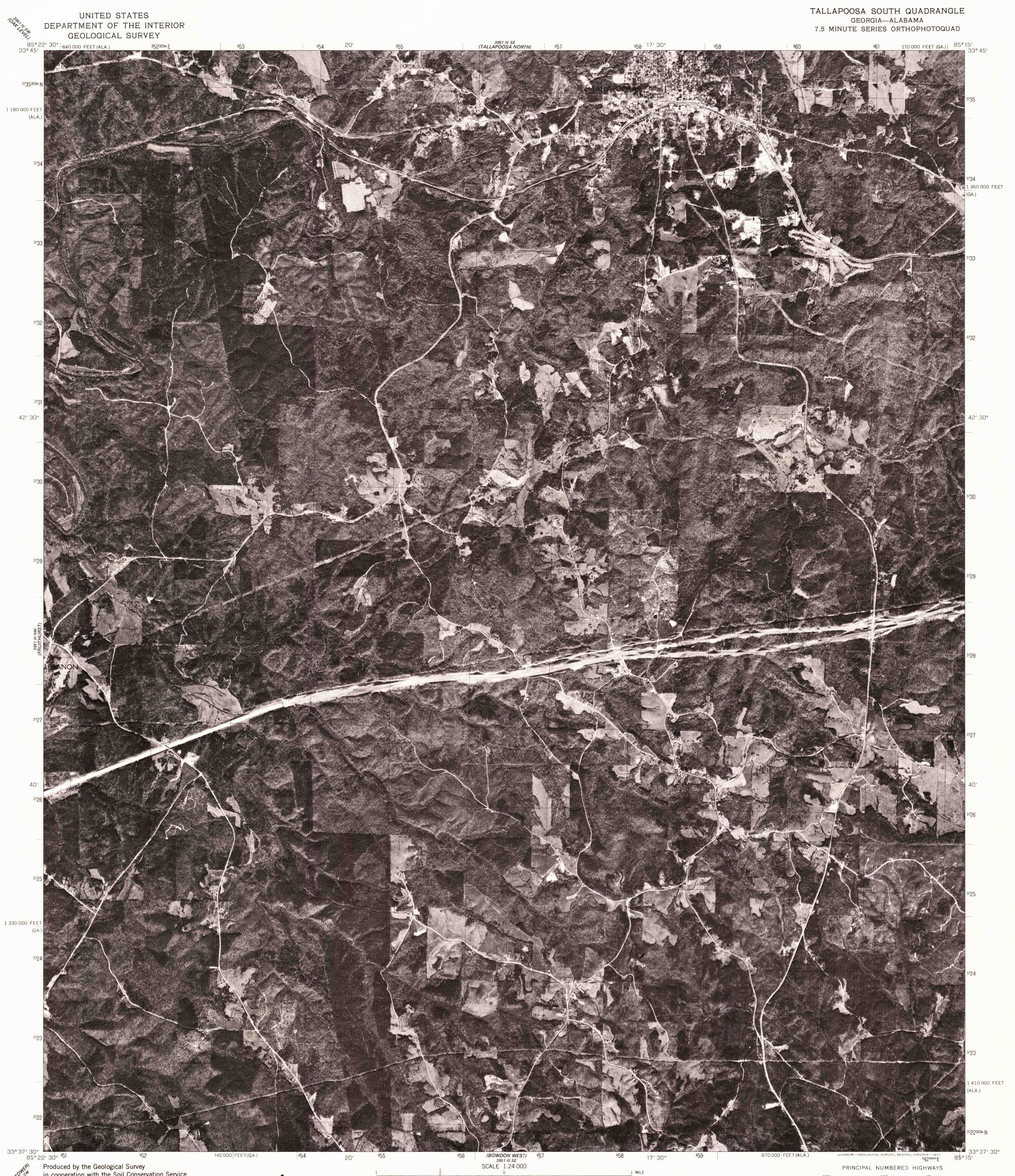
Produced by the Geological Survey in cooperation with the Soil Conservation Service Orthophotograph prepared from 1:76,000-scale aerial photograph taken November 17, 1975
