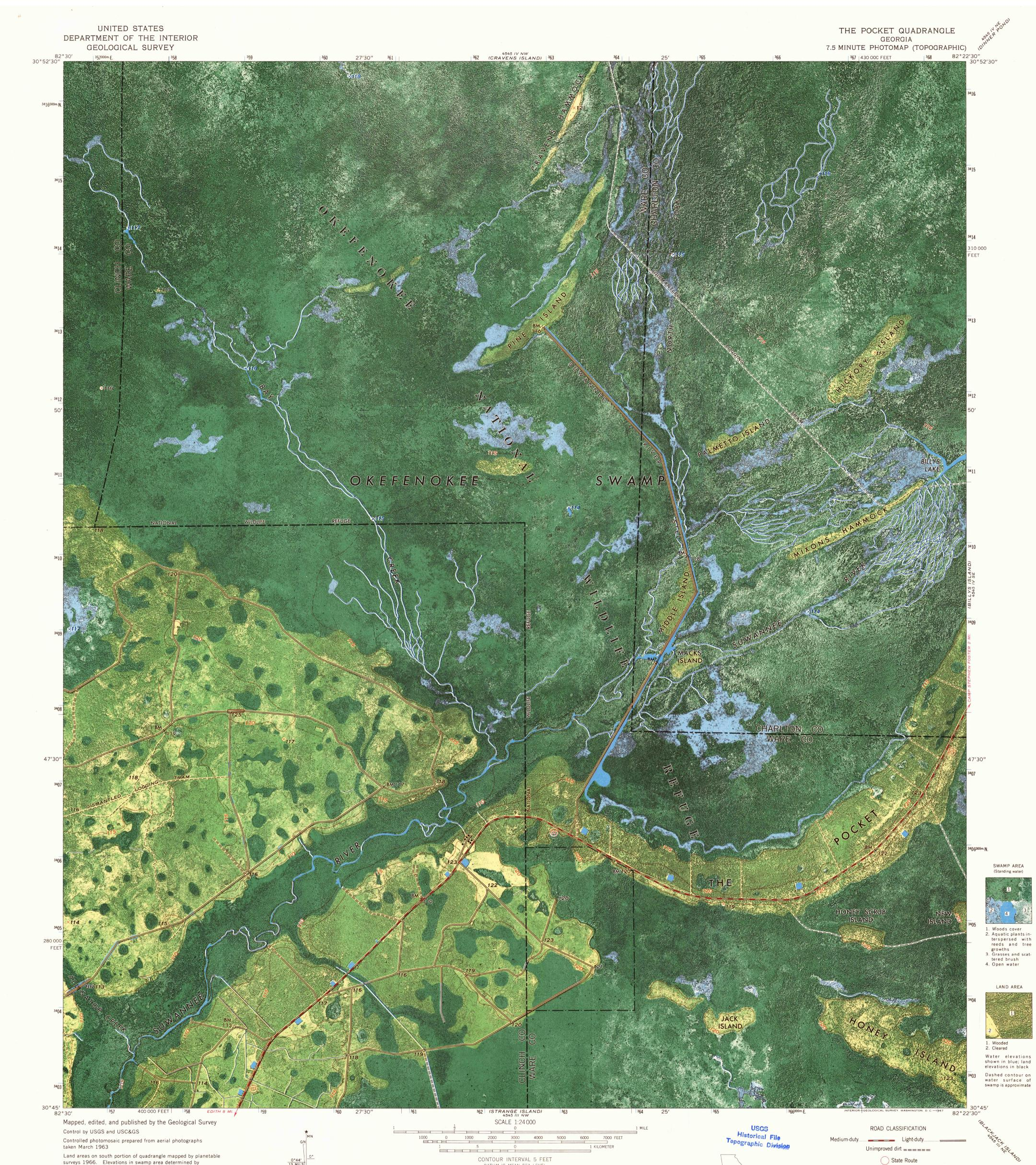
Land areas on south portion of quadrangle mapped by planetable surveys 1966. Elevations in swamp area determined by Air Borne Control System December 1965
