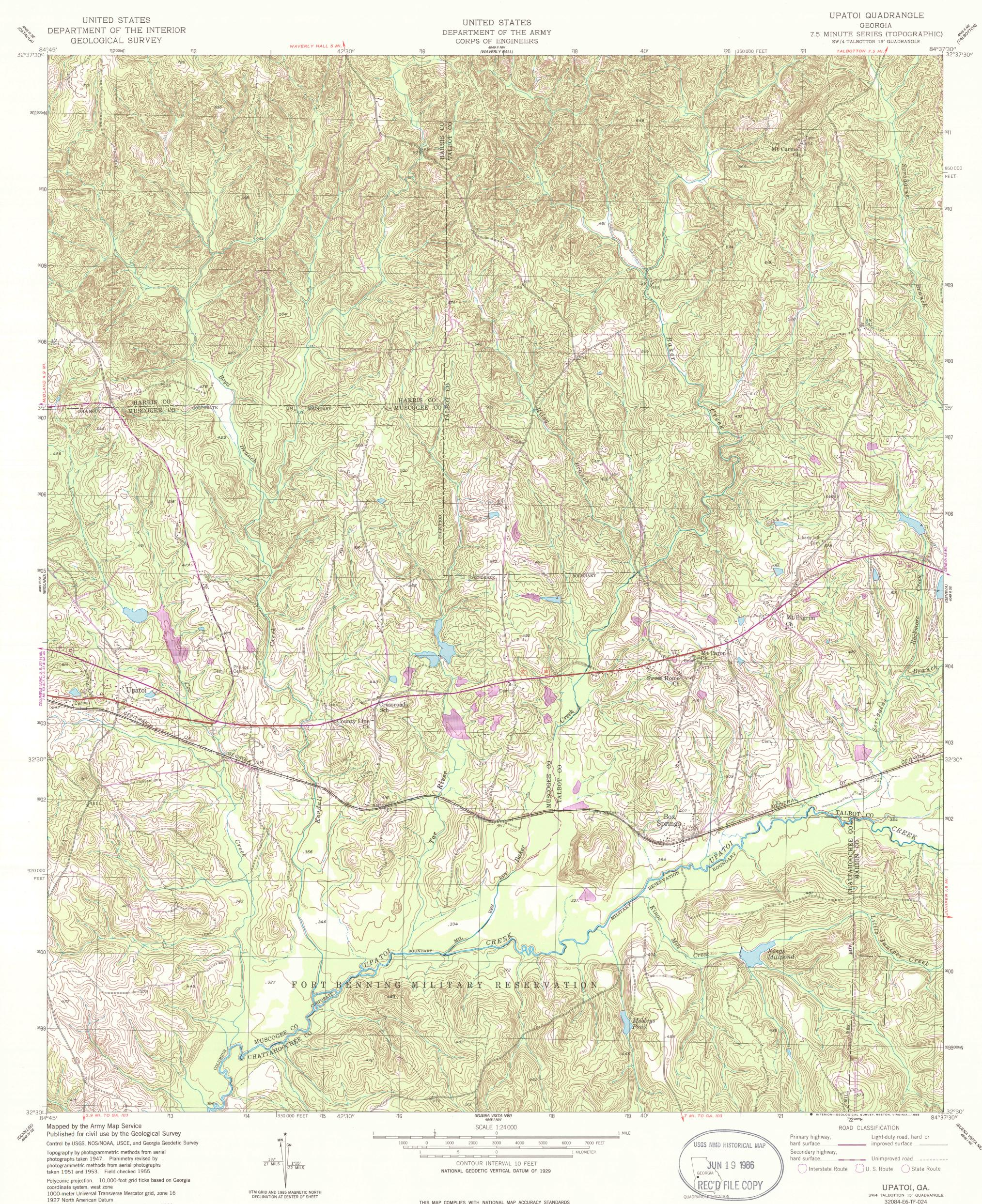
To place on the predicted North American Datum 1983, move the projection lines 13 meters south and 8 meters west as shown by dashed corner ticks
