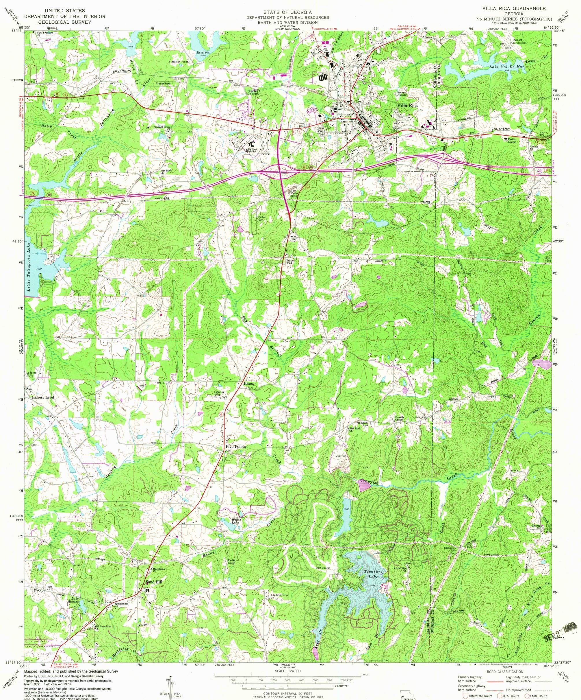
1000-meter Universal Transverse Mercator grid ticks, zone 16, shown in blue. 1927 North American Datum To place on the predicted North American Datum 1983 move the projection lines 10 meters south and 6 meters west as shown by dashed corner ticks
