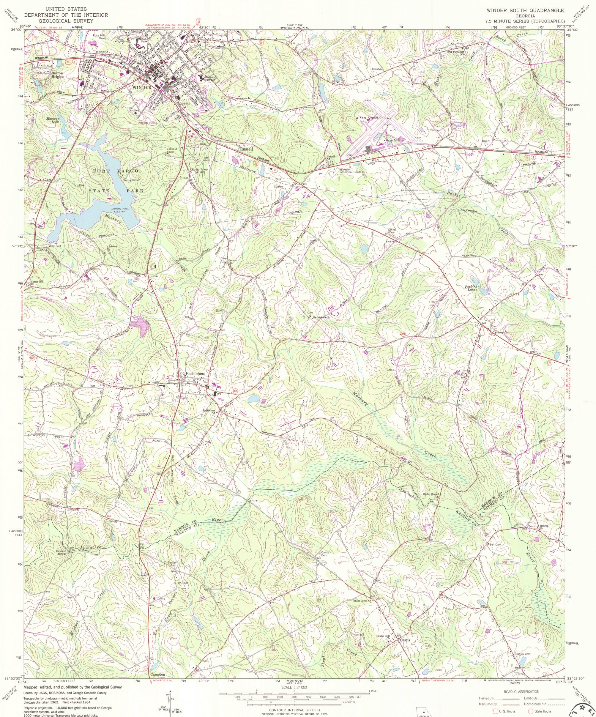
coordinate system, west zone 1000-meter Universal Transverse Mercator grid ticks, zone 17, shown in blue 1927 North American Datum To place on the predicted North American Datum 1983 move the projection lines 11 meters south and 10 meters west as shown by dashed corner ticks Fine red dashed lines indicate selected fence and field lines where
