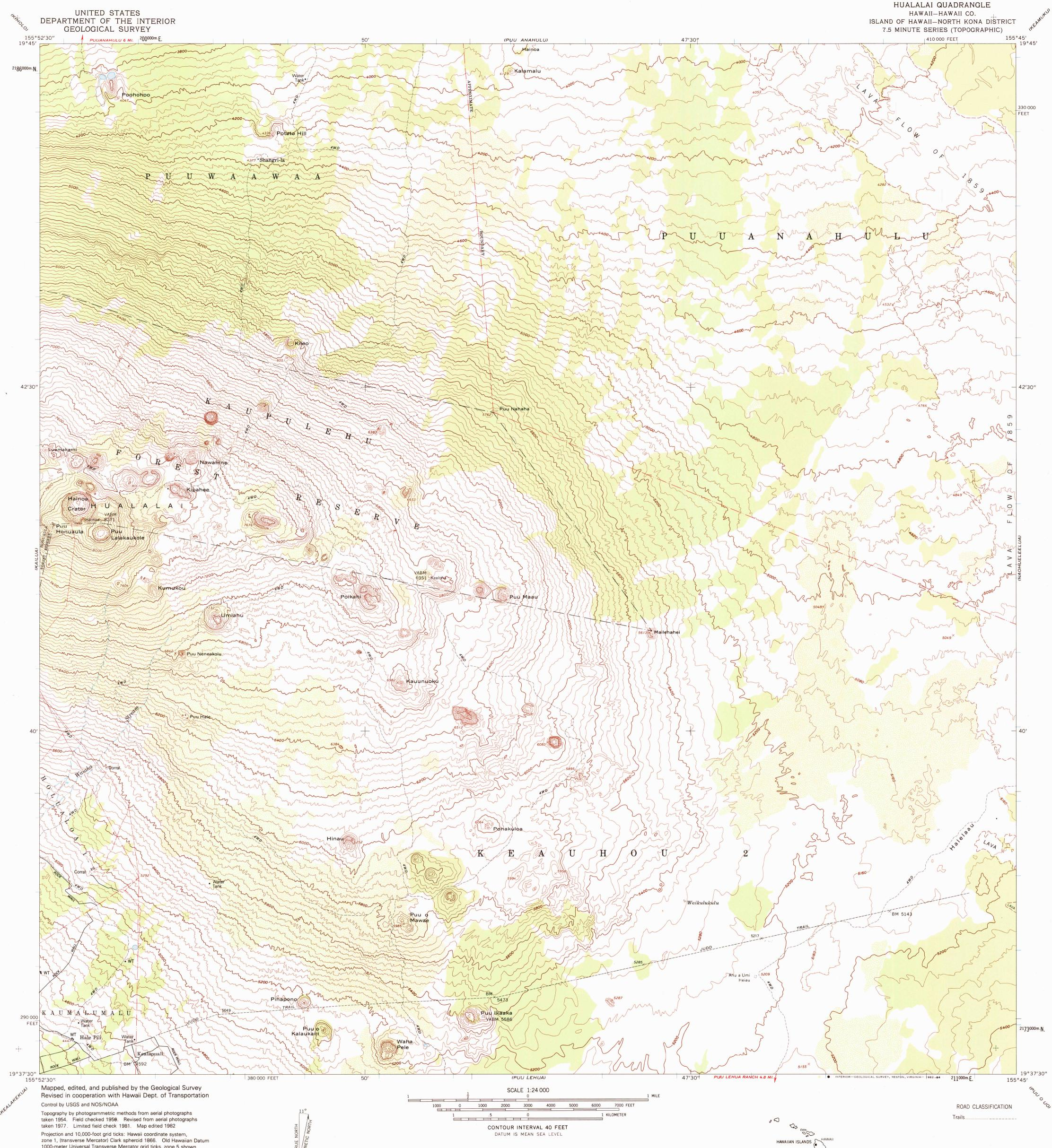
zone 1, (transverse Mercator) Clark spheroid 1866. Old Hawaiian Datum 1000-meter Universal Transverse Mercator grid ticks, zone 5 shown in blue. International spheroid. To place on the predicted North American Datum 1983 move the projection lines 341 meters north and 291 meters west as shown by dashed corner ticks
