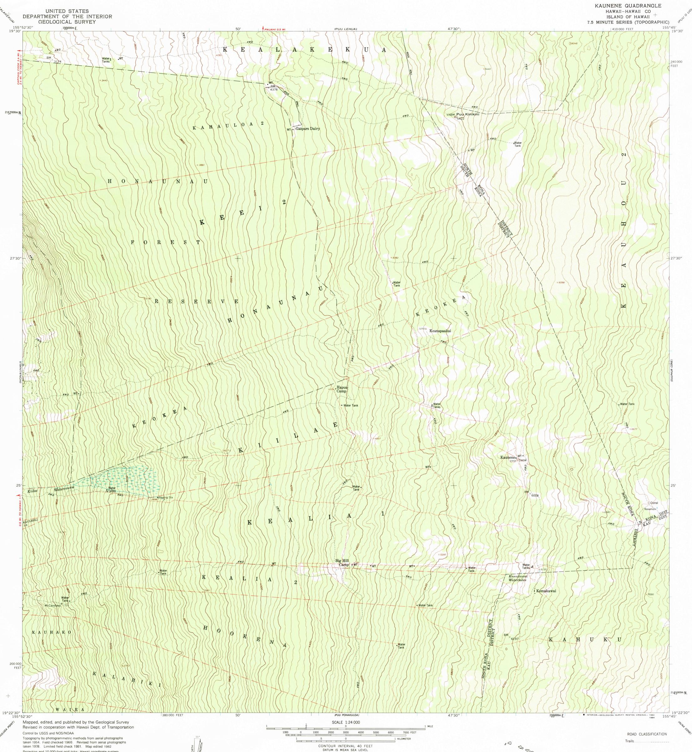
Projection and 10,000-foot grid ticks: Hawaii coordinate system, zone 1 (transverse Mercator) Clark spheroid 1866. Old Hawaiian Datum 1000-meter Universal Transverse Mercator grid ticks, zone 5 shown in blue. International spheroid. To place on the predicted North American Datum 1983 move the projection lines 338 meters north and 291 meters west as shown by dashed corner ticks
