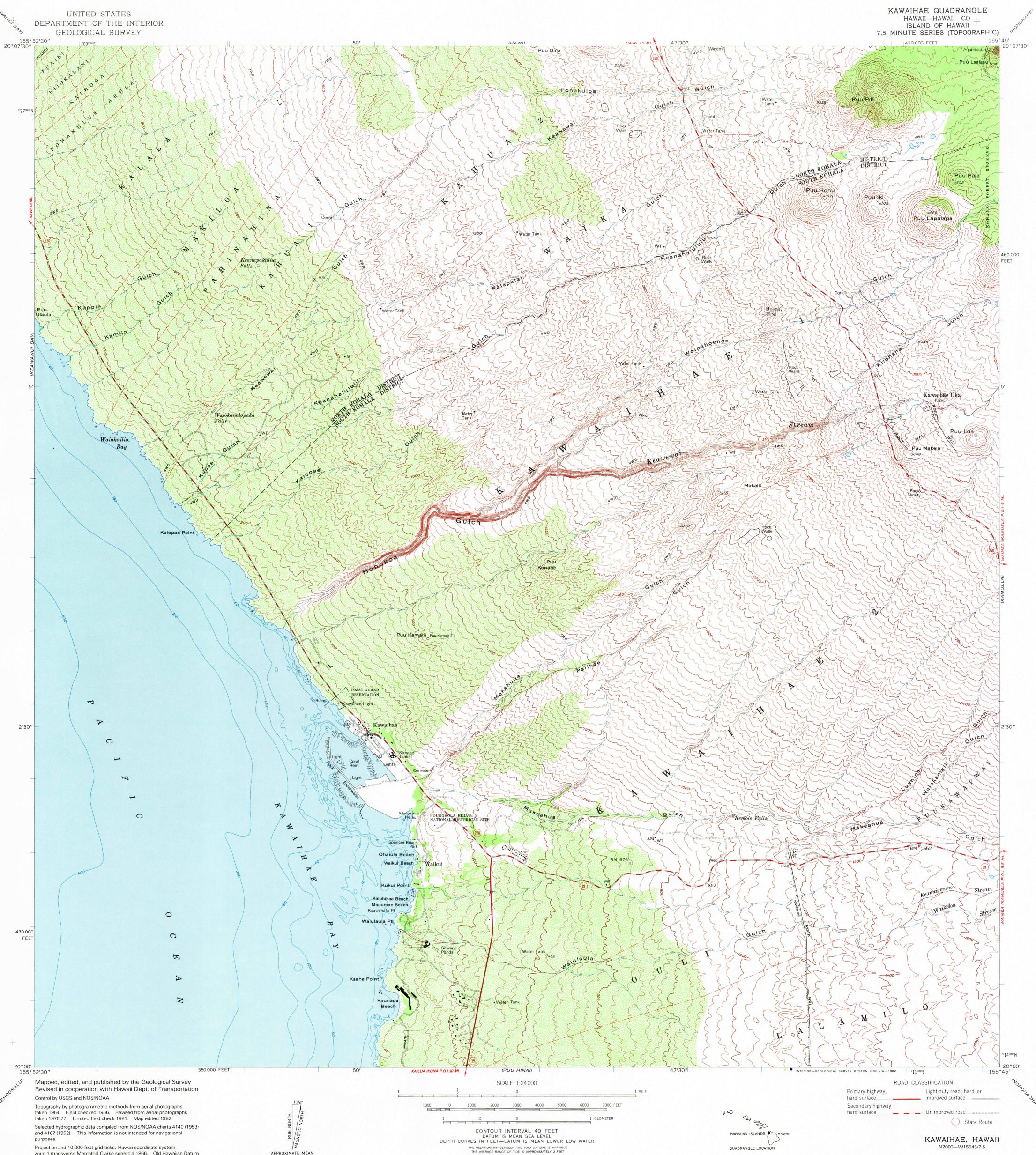
Projection and 10,000-foot grid ticks: Hawaii coordinate system, zone 1 (transverse Mercator) Clarke spheroid 1866. Old Hawaiian Datum 1000-meter Universal Transverse Mercator grid ticks, zone 5, shown in blue. International spheroid. To place on the predicted North American Datum 1983 move the projection lines 344 meters north and 292 meters west as shown by dashed corner ticks There may be private inholdings within the boundaries of the National or State reservations shown on this map
