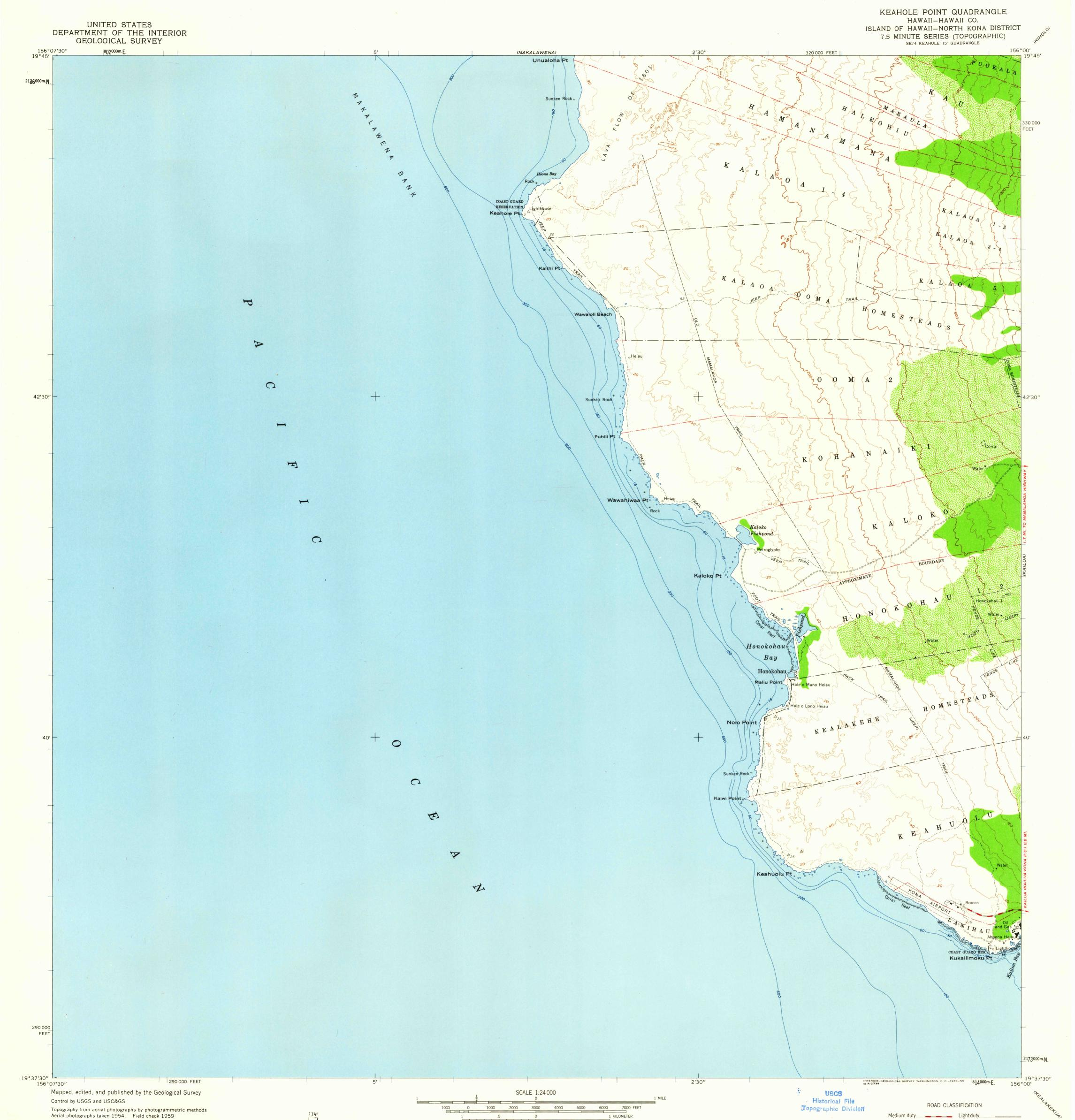
Hydrography compiled from USC&GS charts 4140 (1953) and 4164 (1951) Polyconic projection. Old Hawaiian datum 10,000-foot grid based on Hawaiian coordinate system, zone 1 1000-meter Universal Transverse Mercator grid ticks, zone 4, shown in blue CONTOUR INTERVAL 40 FEET DOTTED LINES REPRESENT 20-FOOT CONTOURS DATUM IS MEAN SEA LEVEL DEPTH CURVES IN FEET—DATUM IS MEAN LOWER LOW WATER SHORELINE SHOWN REPRESENTS THE APPROXIMATE LINE OF MEAN HIGH WATER THE MEAN RANGE OF TIDE IS APPROXIMATELY 1 FOOT
