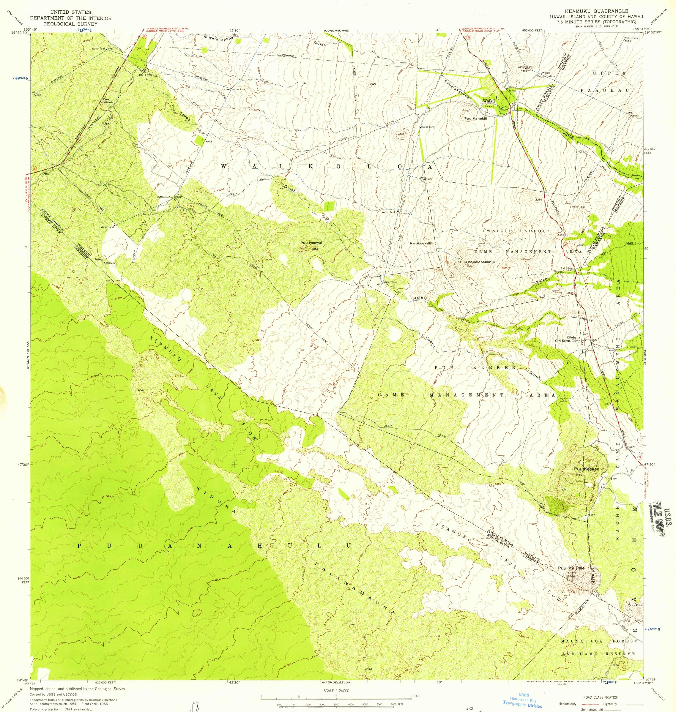
Polyconic projection. Old Hawaiian datum 10,000-foot grid based on Hawaiian coordinate system, zone 1
