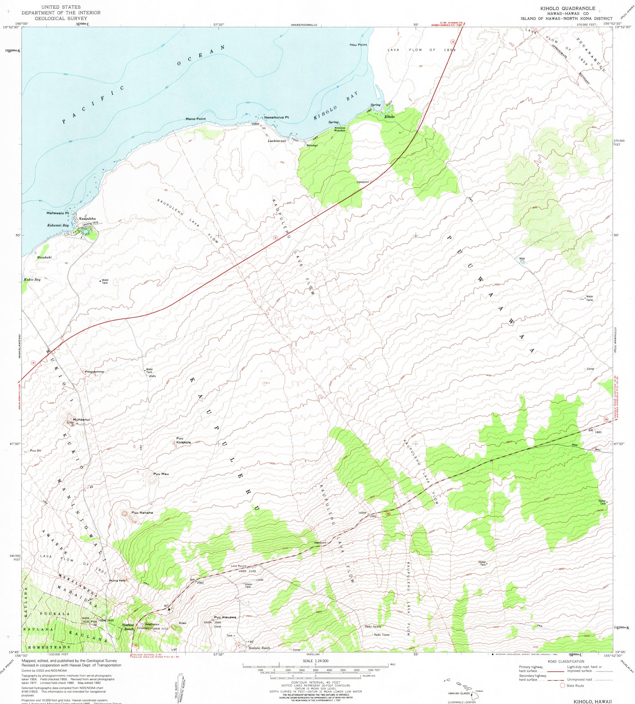
Projection and 10,000-foot grid ticks: Hawaii coordinate system, zone 1 (transverse Mercator) Clarke spheroid 1866. Old Hawaiian Datum 1000-meter Universal Transverse Mercator grid ticks, zone 5, shown in blue. International spheroid. To place on the predicted North American Datum 1983 move the projection lines 343 meters north and 291 meters west as shown by dashed corner ticks
