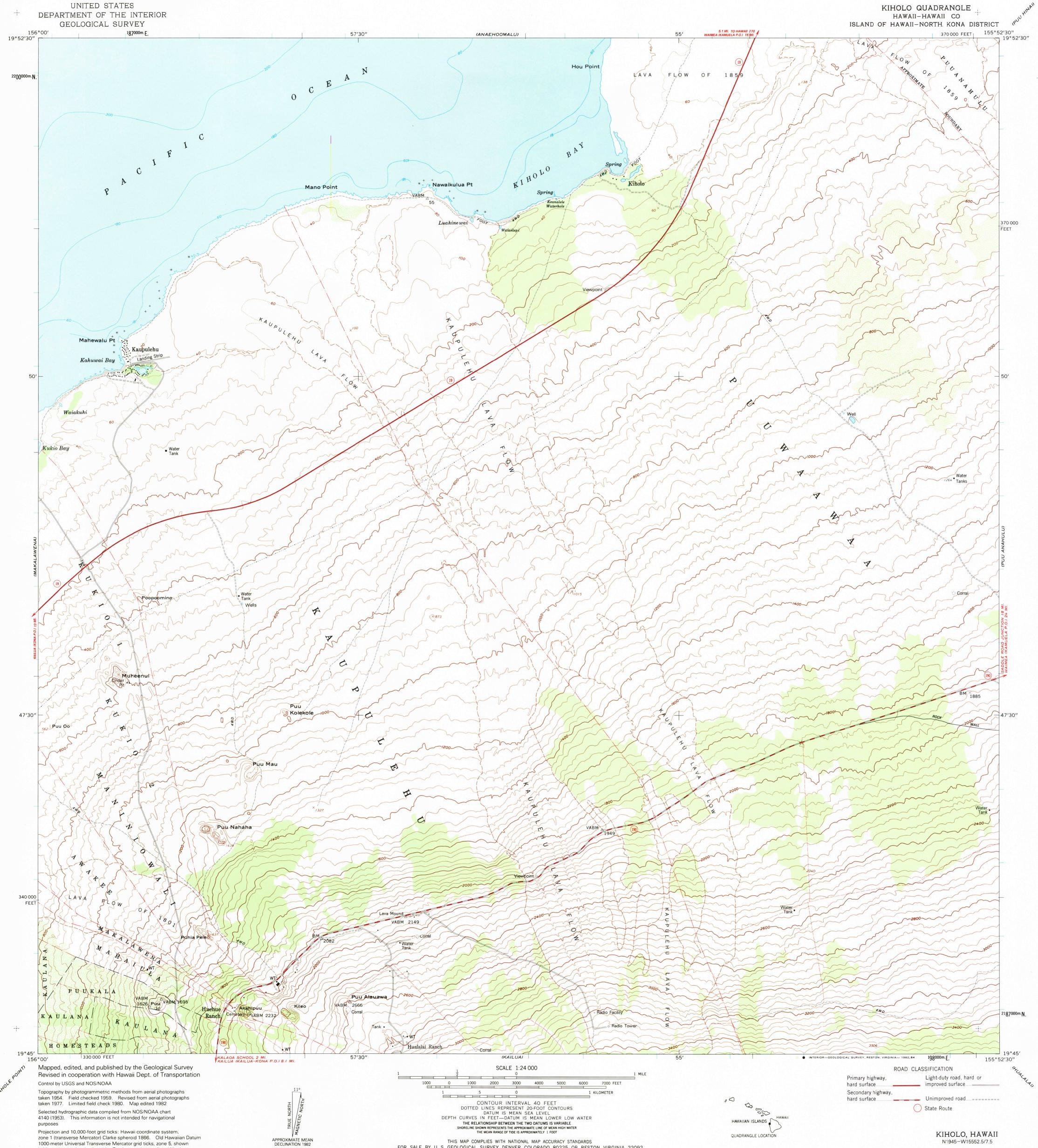
1000-meter Universal Transverse Mercator grid ticks, zone 5, shown in blue. International spheroid. To place on the predicted North American Datum 1983 move the projection lines 343 meters north and 291 meters west as shown by dashed corner ticks
