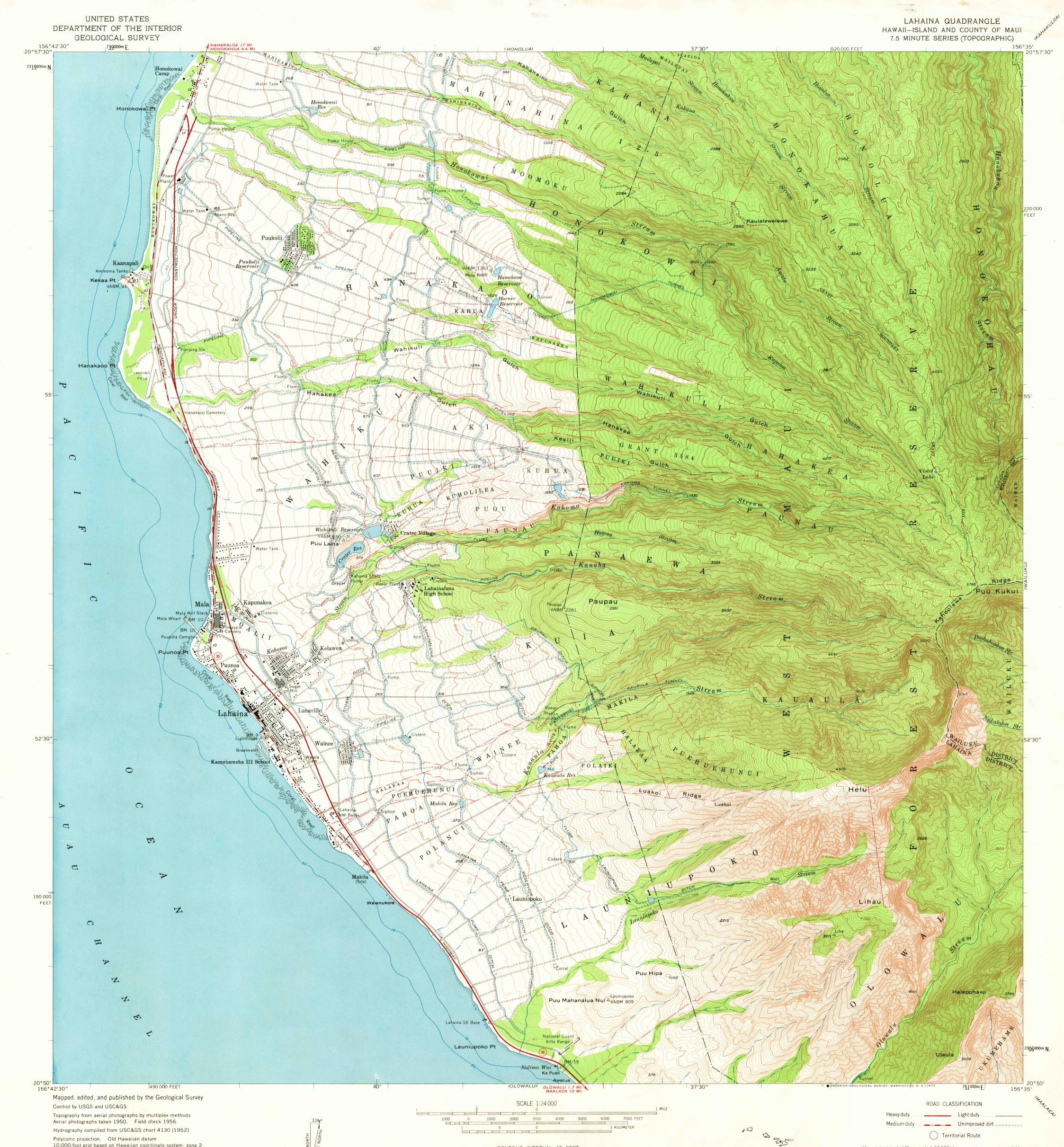
Polyconic projection. Old Hawaiian datum 10,000-foot grid based on Hawaiian coordinate system, zone 2 1000-meter Universal Transverse Mercator grid ticks, zone 4, shown in blue
