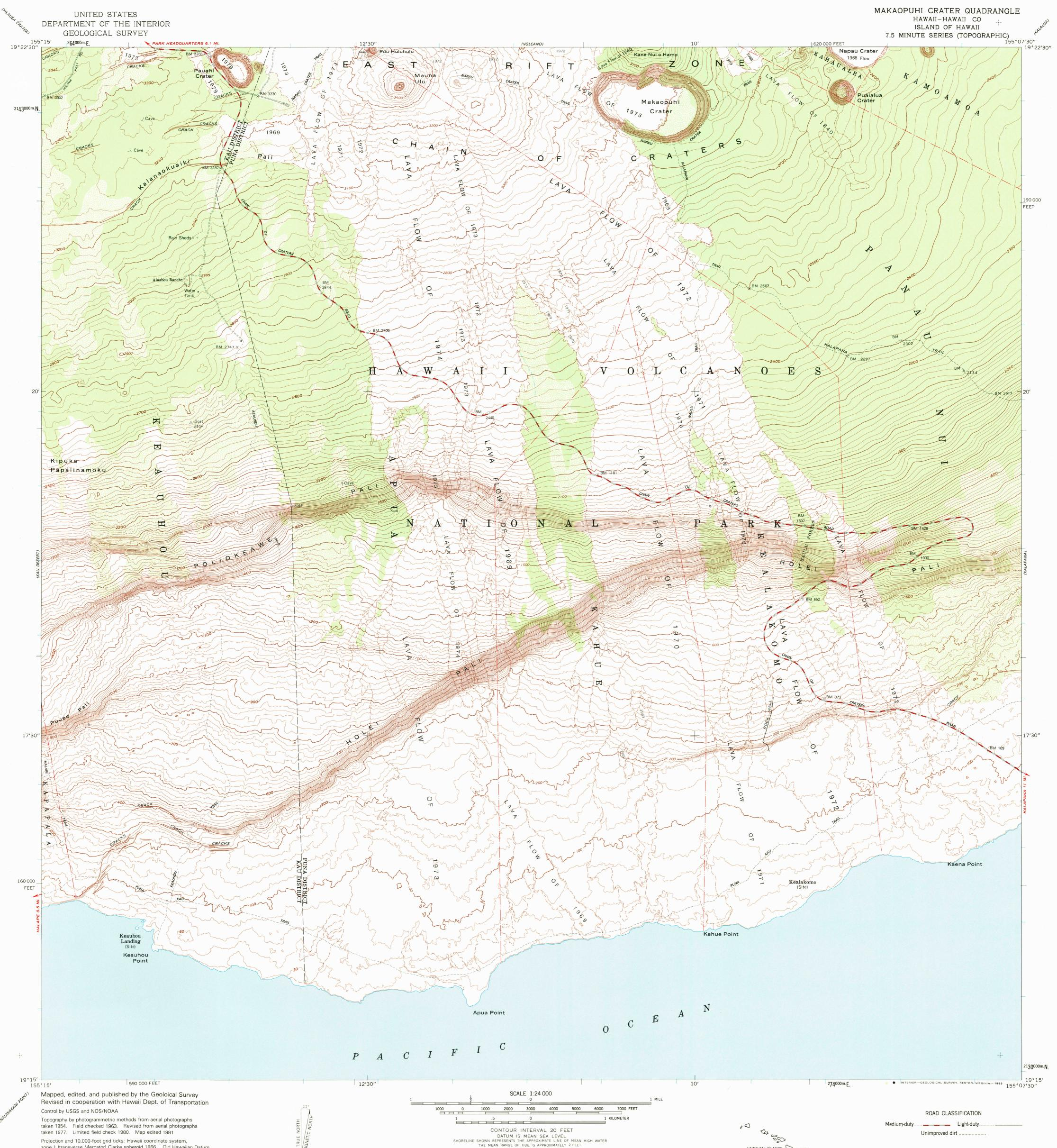
Projection and 10,000-foot grid ticks: Hawaii coordinate system, zone 1 (transverse Mercator) Clarke spheroid 1866. Old Hawaiian Datum 1000-meter Universal Transverse Mercator grid ticks, zone 5 shown in blue. International spheroid. To place on the predicted North American Datum 1983 move the projection line 337 meters north and 291 meters west as shown by dashed corner ticks
