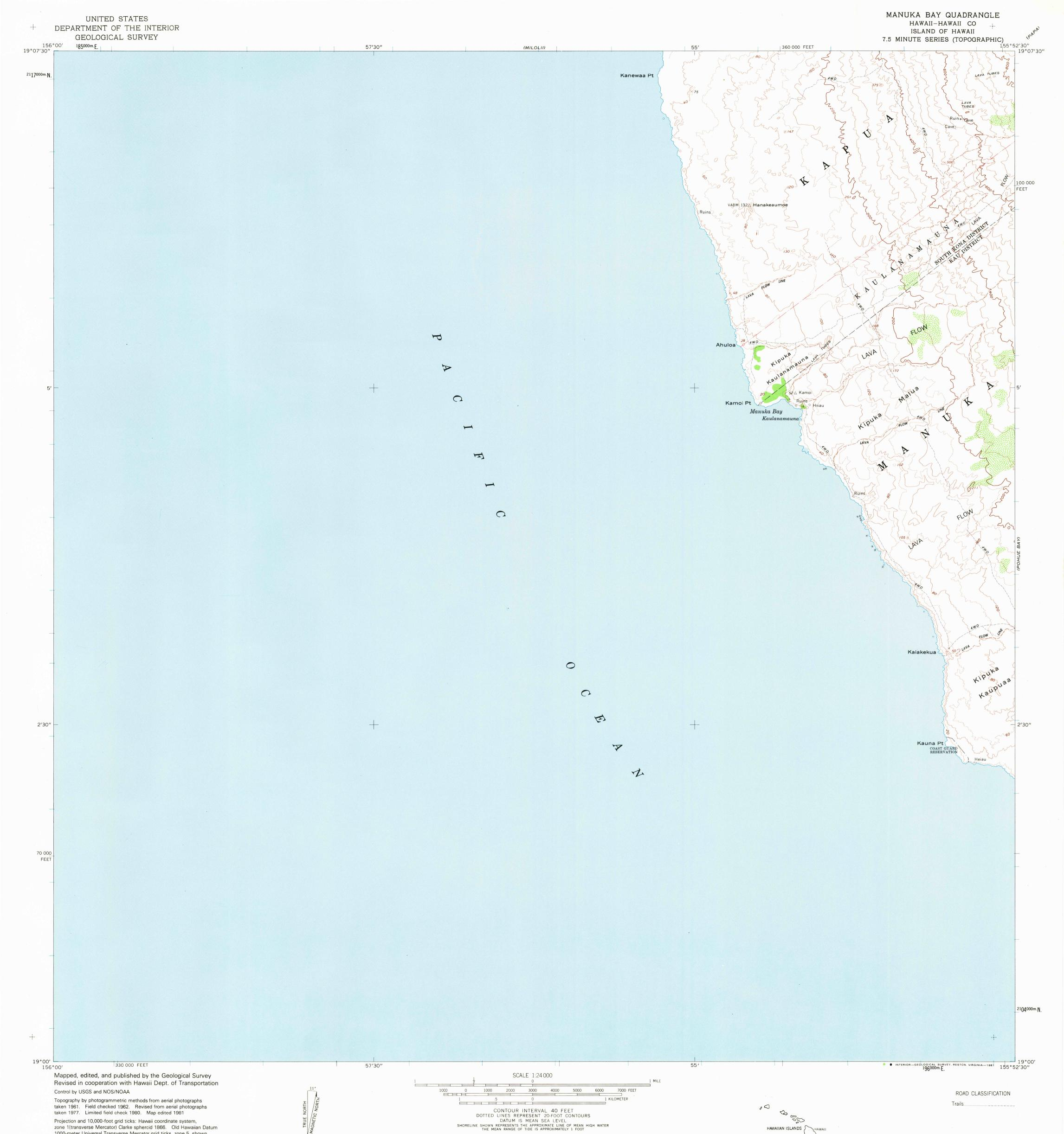
Projection and 10,000-foot grid ticks: Hawaii coordinate system, zone 1(transverse Mercator) Clarke sphercid 1866. Old Hawaiian Datum 1000-meter Universal Transverse Mercator grid ticks, zone 5, shown in blue. International spheroid. To place on the predicted North American Datum 1983 move the projection lines 335 meters north and 291 meters west as shown by dashed corner ticks There may be private inholdings within the boundaries of the National or State reservations shown on this map
