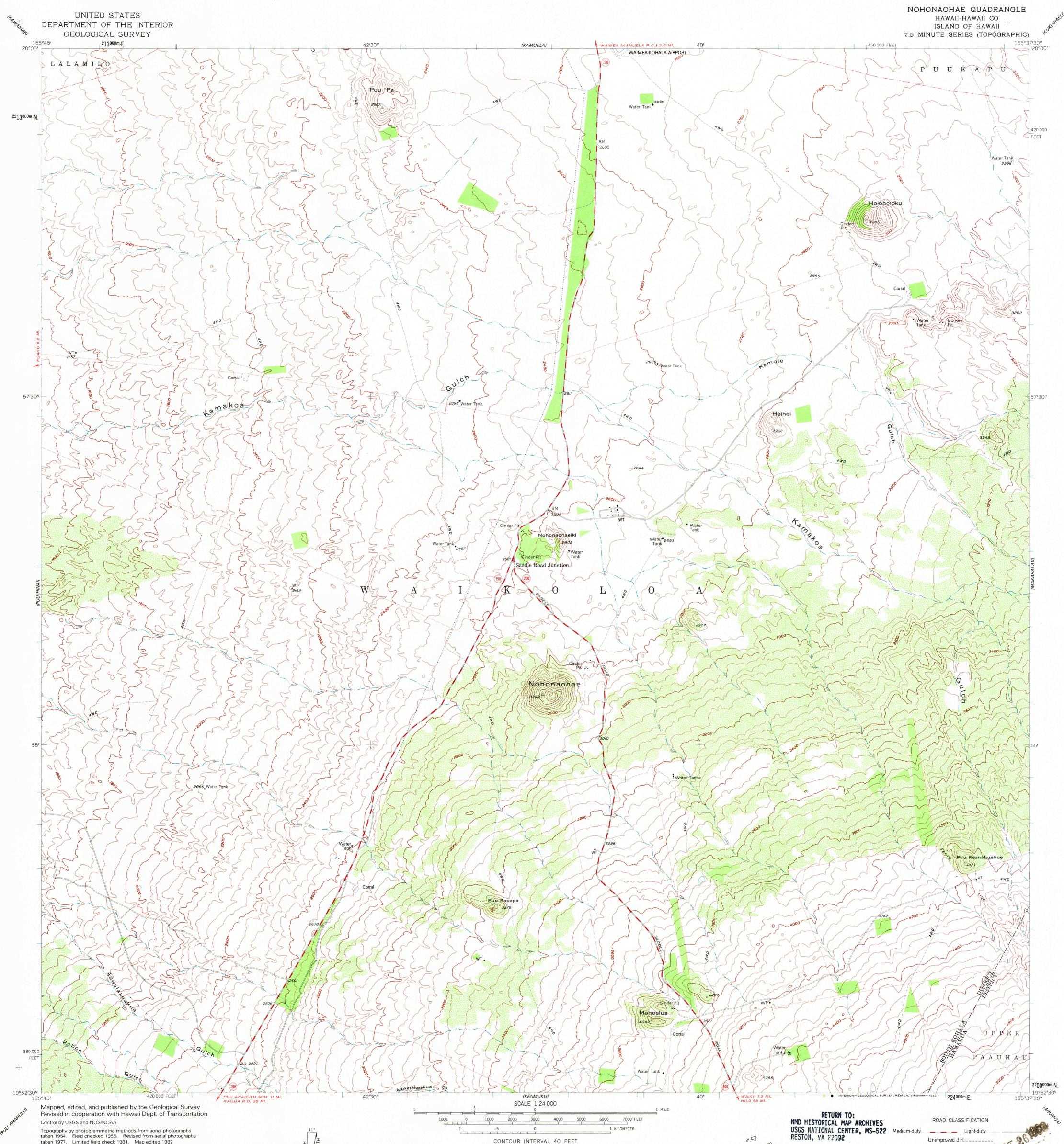
Projection and 10,000-foot grid ticks: Hawaii coordinate system, zone 1 (transverse Mercator) Clarke spheroid 1866. Old Hawaiian Datum 1000-meter Universal Transverse Mercator grid ticks, zone 5 shown in blue. International spheroid. To place on the predicted North American Datum 1983 move the projection lines 343 meters north and 292 meters west as shown by dashed corner ticks
