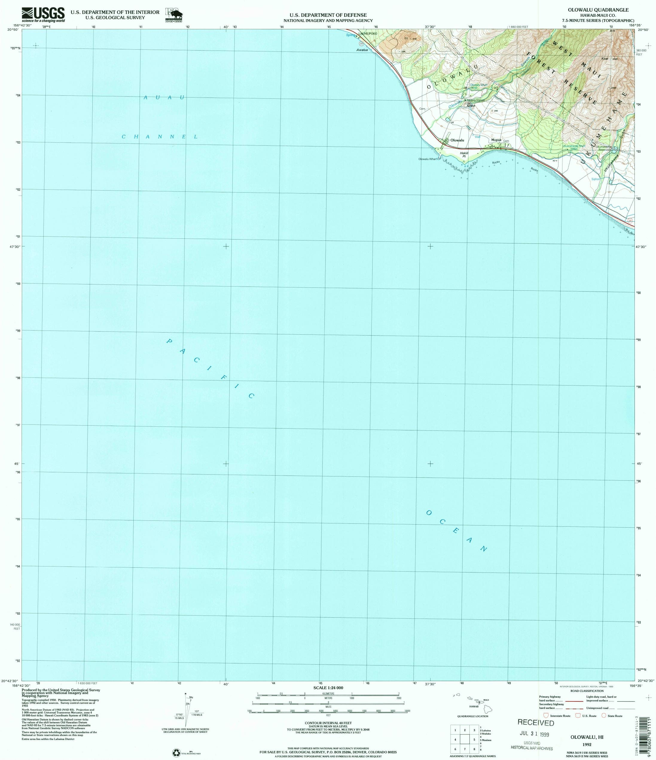
10 000-foot ticks: Hawaii Coordinate System of 1983 (zone 2) Old Hawaiian Datum is shown by dashed corner ticks The values of the shift between Old Hawaiian Datum and NAD 83 for 7.5-minute intersections are obtainable from National Geodetic Survey NADCON software
