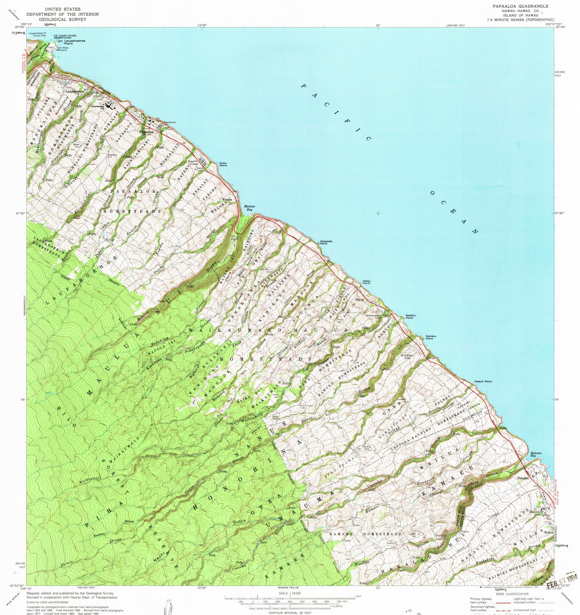
Projection and 10,000-foot grid ticks: Hawaii coordinate system, zone 1 (transverse Mercator) Clark spheroid 1866. Old Hawaiian Datum 1000-meter Universal Transverse Mercator grid ticks, zone 5 shown in blue. International spheroid. To place on the predicted North American Datum 1983 move the projection lines 341 meters north and 291 meters west as shown by dashed corner ticks
