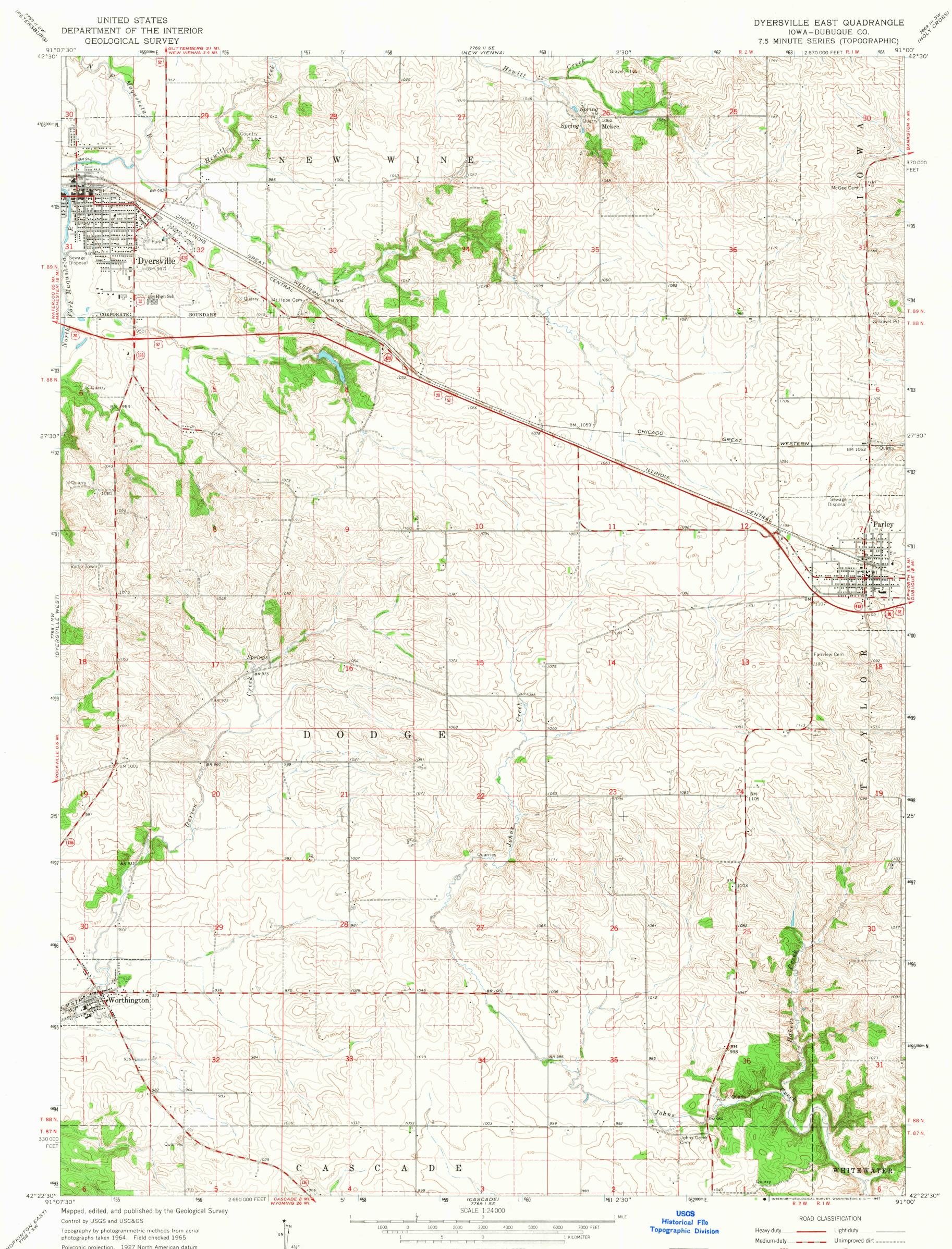
Polyconic projection. 1927 North American datum 10,000-foot grid based on Iowa coordinate system, north zone 1000-meter Universal Transverse Mercator grid ticks, zone 15, shown in blue
