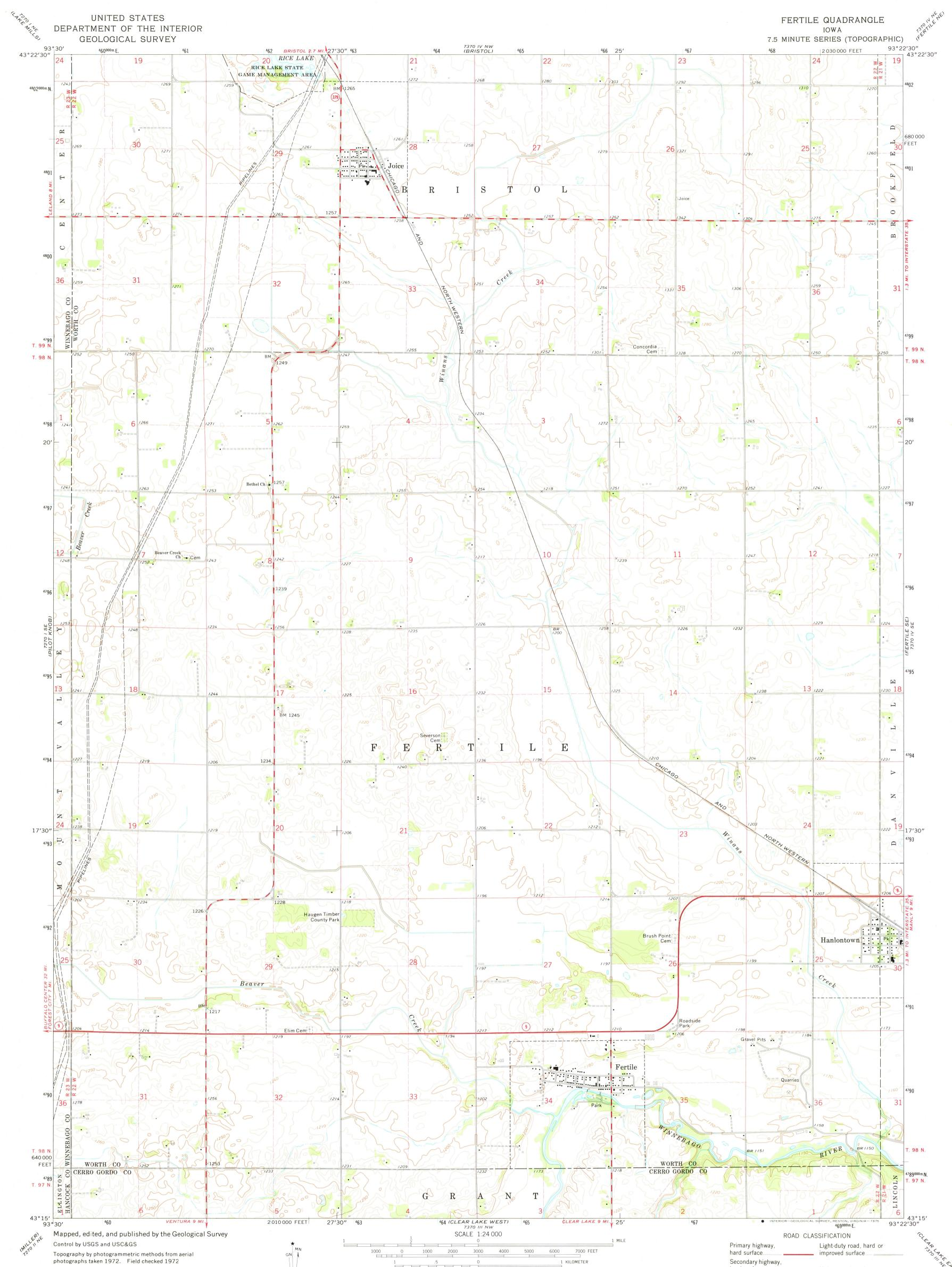
Projection and 10,000-foot grid ticks: Iowa coordinate system, north zone (Lambert conformal conic) 1000-meter Universal Transverse Mercator grid ticks, zone 15, shown in blue. 1927 North American datum
