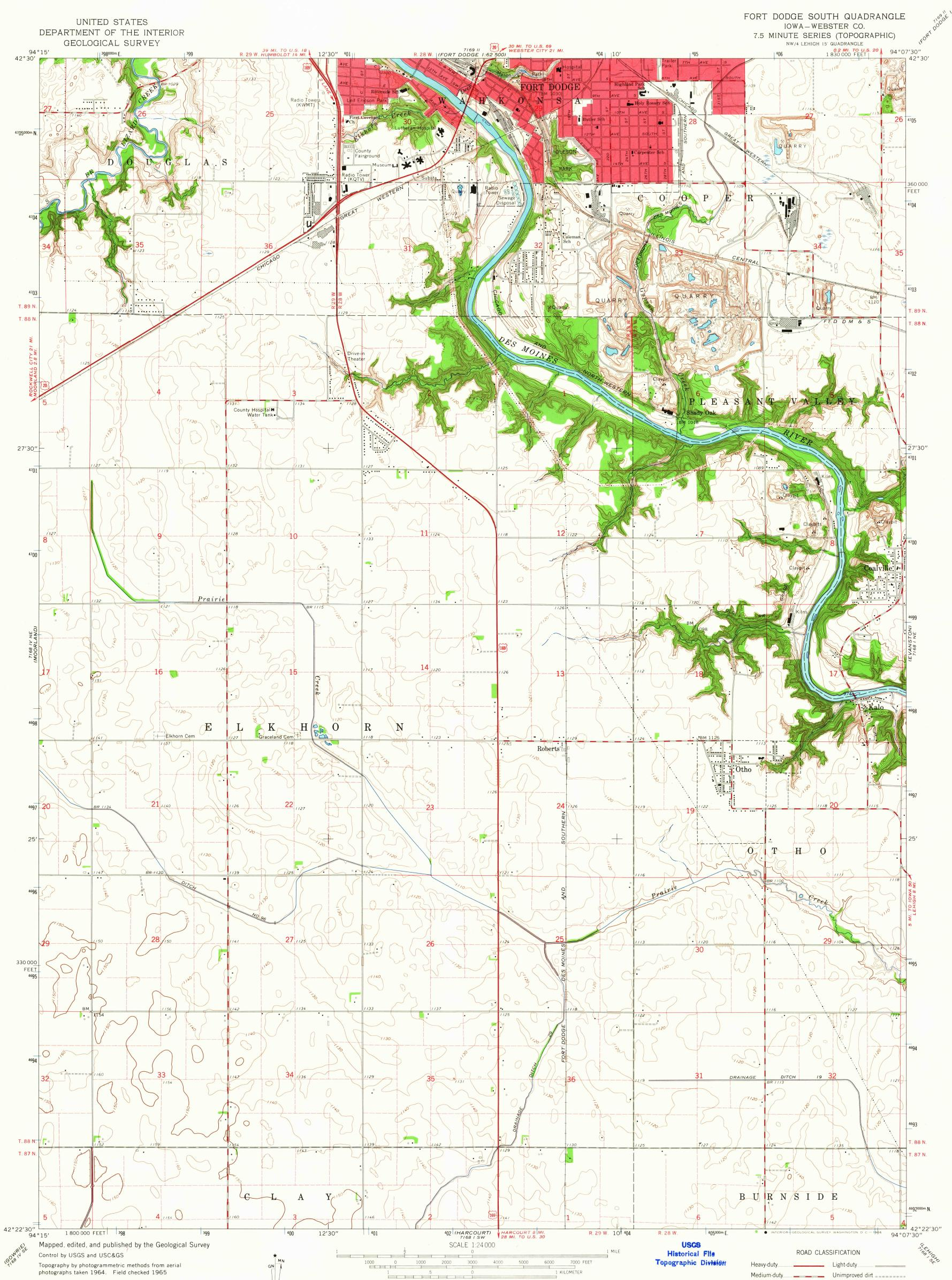
Polyconic projection. 1927 North American datum 10,000-foot grid based on Iowa coordinate system, north zone 1000-meter Universal Transverse Mercator grid ticks, zone 15, shown in blue Red tint indicates areas in which only landmark buildings are shown UTM GRID AND 1965 MAGNETIC NORTH DECLINATION AT CENTER OF SHEET
