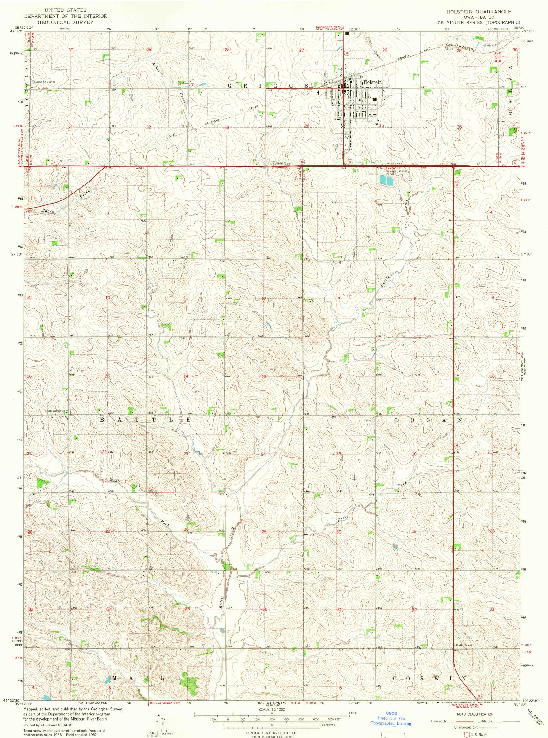
photographs taken 1966. Field checked 1967 Polyconic projection. 1927 North American datum 10.000-foot grid based on Iowa coordinate system, north zone 1000-meter Universal Transverse Mercator grid ticks, zone 15, shown in blue
