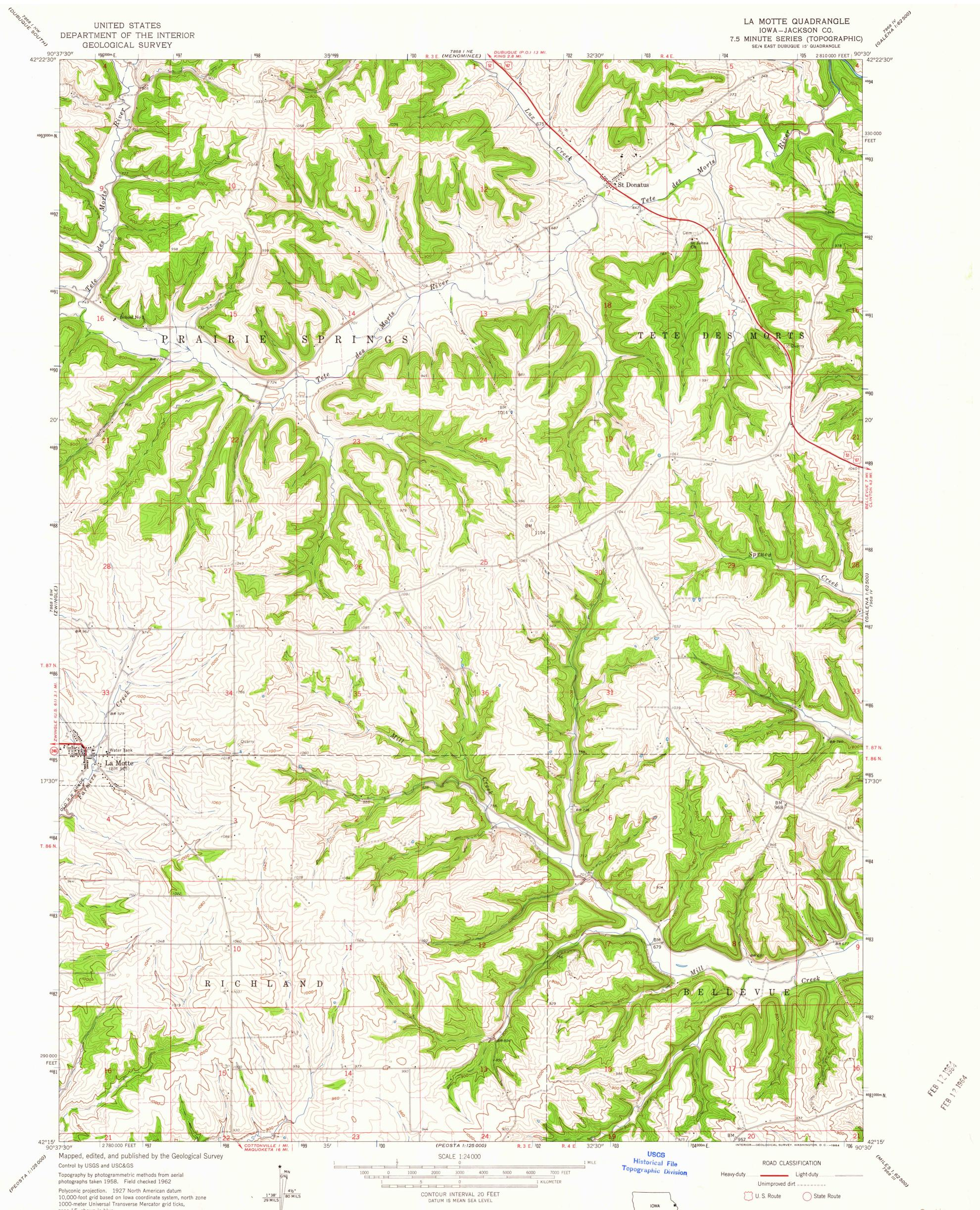
Polyconic projection. 1927 North American datum 10,000-foot grid based on Iowa coordinate system, north zone 1000-meter Universal Transverse Mercator grid ticks, zone 15, shown in blue
