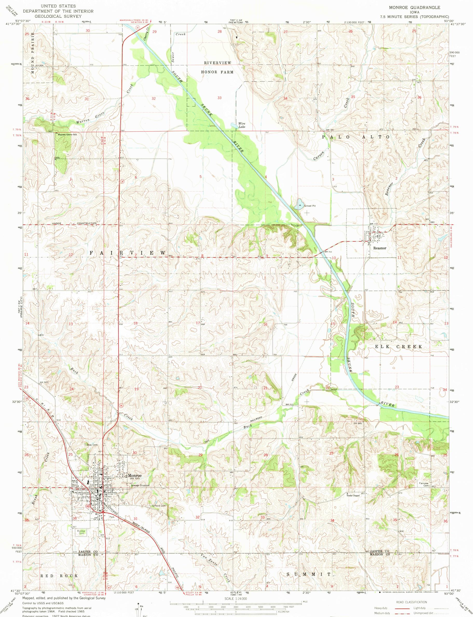
Polyconic projection. 1927 North American datum 10,000-foot grid based on Iowa coordinate system, south zone 1000-meter Universal Transverse Mercator grid ticks, zone 15, shown in blue To place on the predicted North American Datum 1983 move the projection lines 3 meters north and 17 meters east as shown by dashed corner ticks
