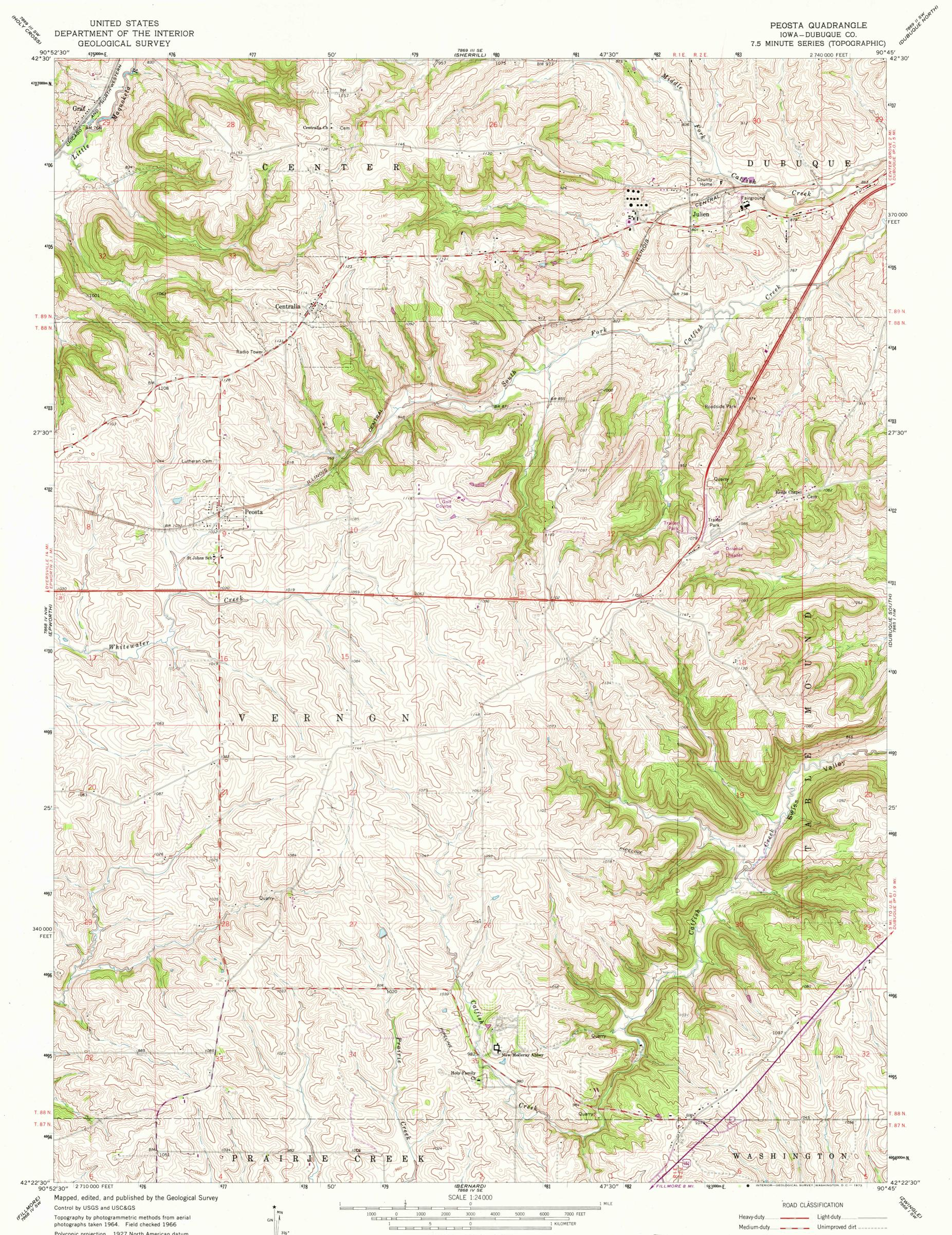
Polyconic projection. 1927 North American datum 10,000-foot grid based on Iowa coordinate system, north zone 1000-meter Universal Transverse Mercator grid ticks, zone 15, shown in blue Fine red dashed lines indicate selected fence and field lines where
