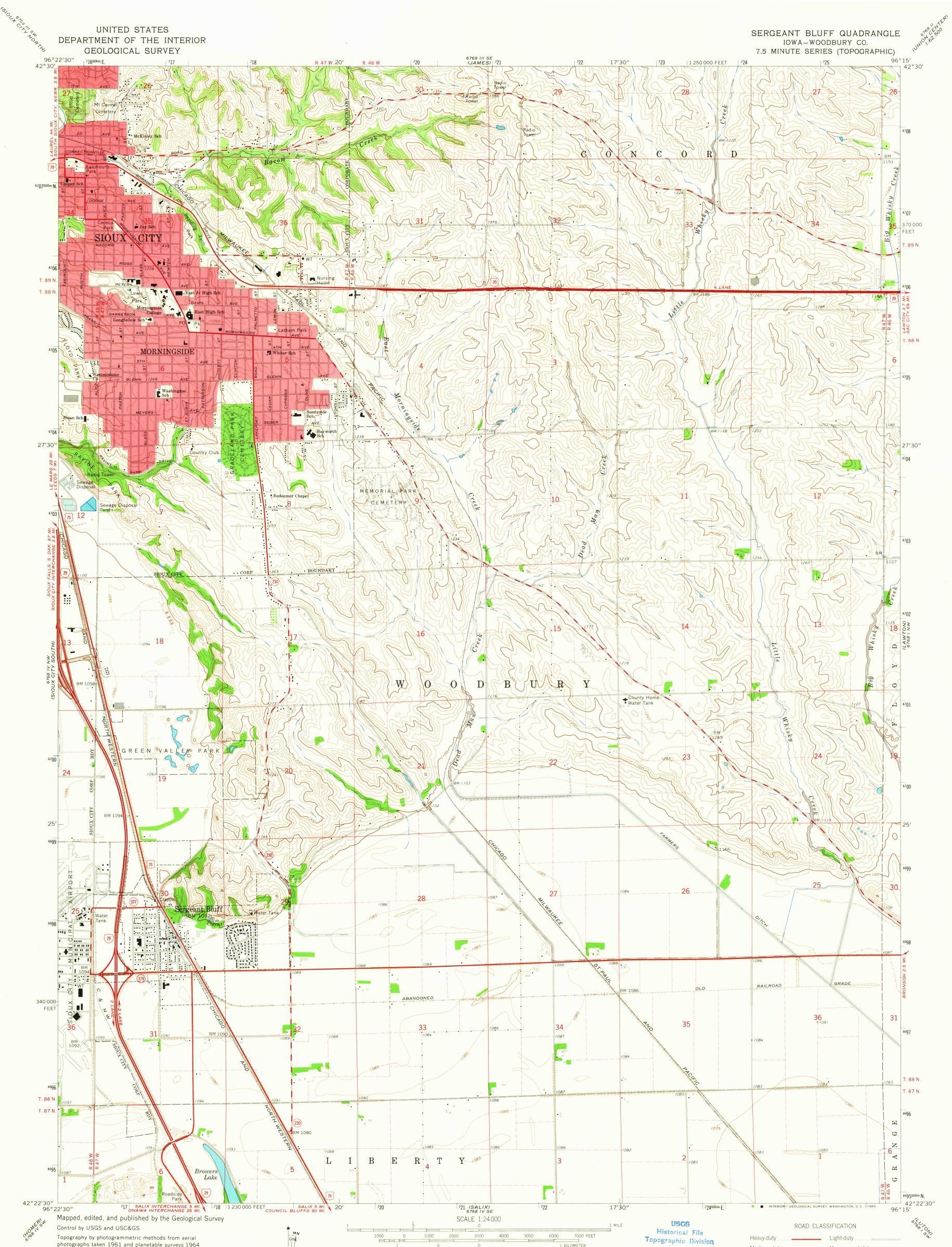
Polyconic projection. 1927 North American datum 10,000-foot grid based on Iowa coordinate system, north zone 1000-meter Universal Transverse Mercator grid ticks, zone 14, shown in blue
