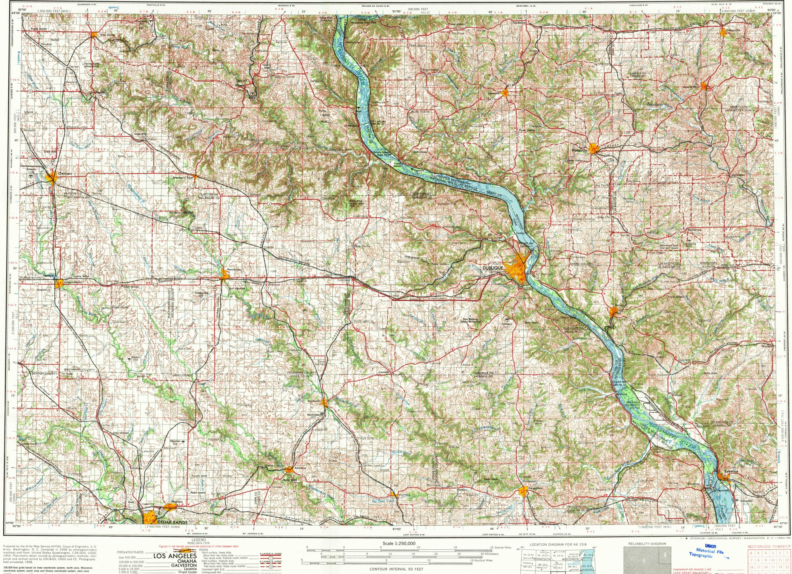
100,000-foot grids based on lowa coordinate system, north zone, Wisconsin coordinate system, south zone and Illinois coordinate system, west zone 10,000-meter Universal Transverse Mercator grid ticks, zone 15, shown in blue
