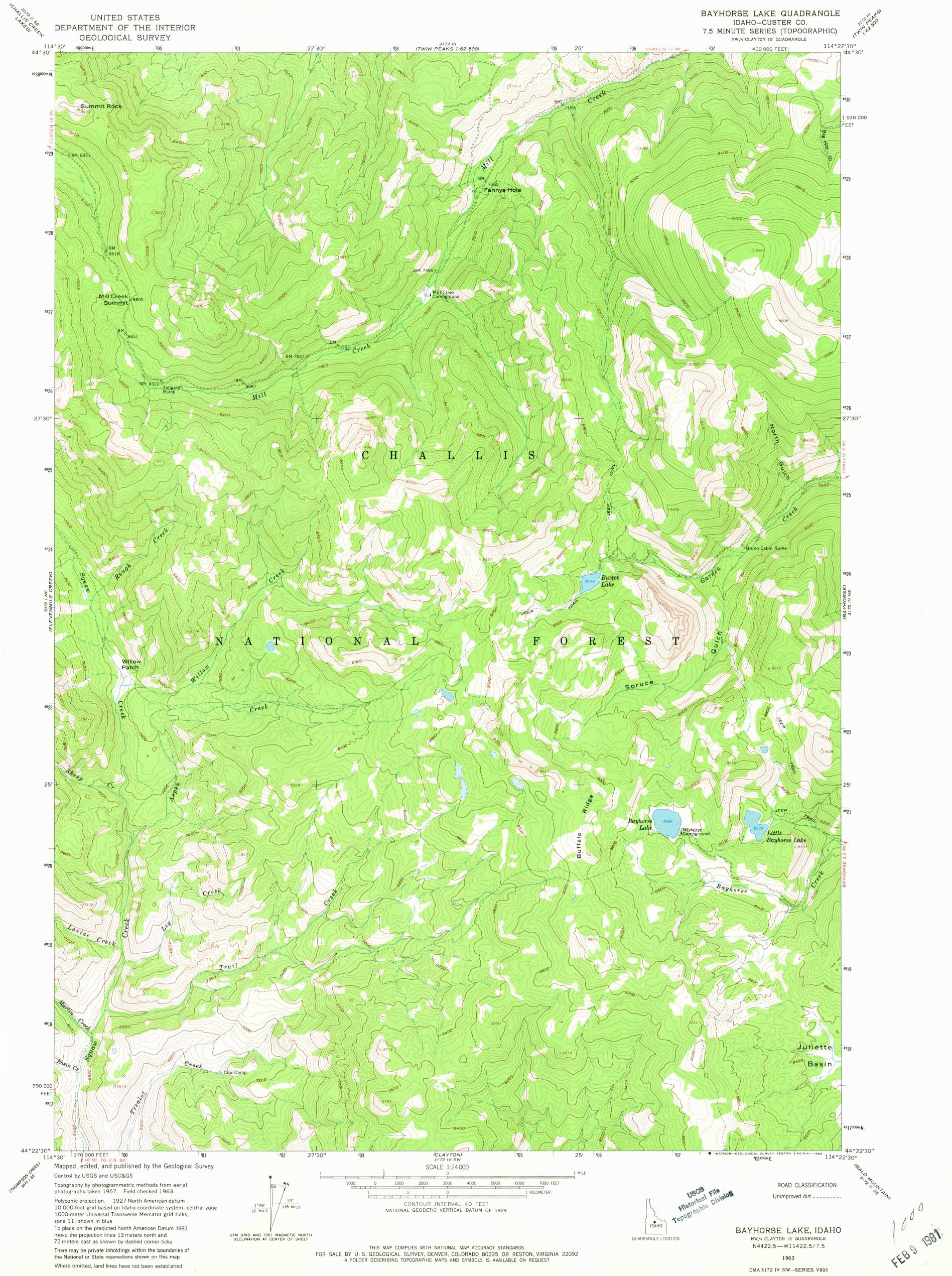
10,000-foot grid based on Idaho coordinate system, central zone 1000-meter Universal Transverse Mercator grid ticks, zone 11, shown in blue To place on the predicted North American Datum 1983 move the projection lines 13 meters north and 72 meters east as shown by dashed corner ticks
