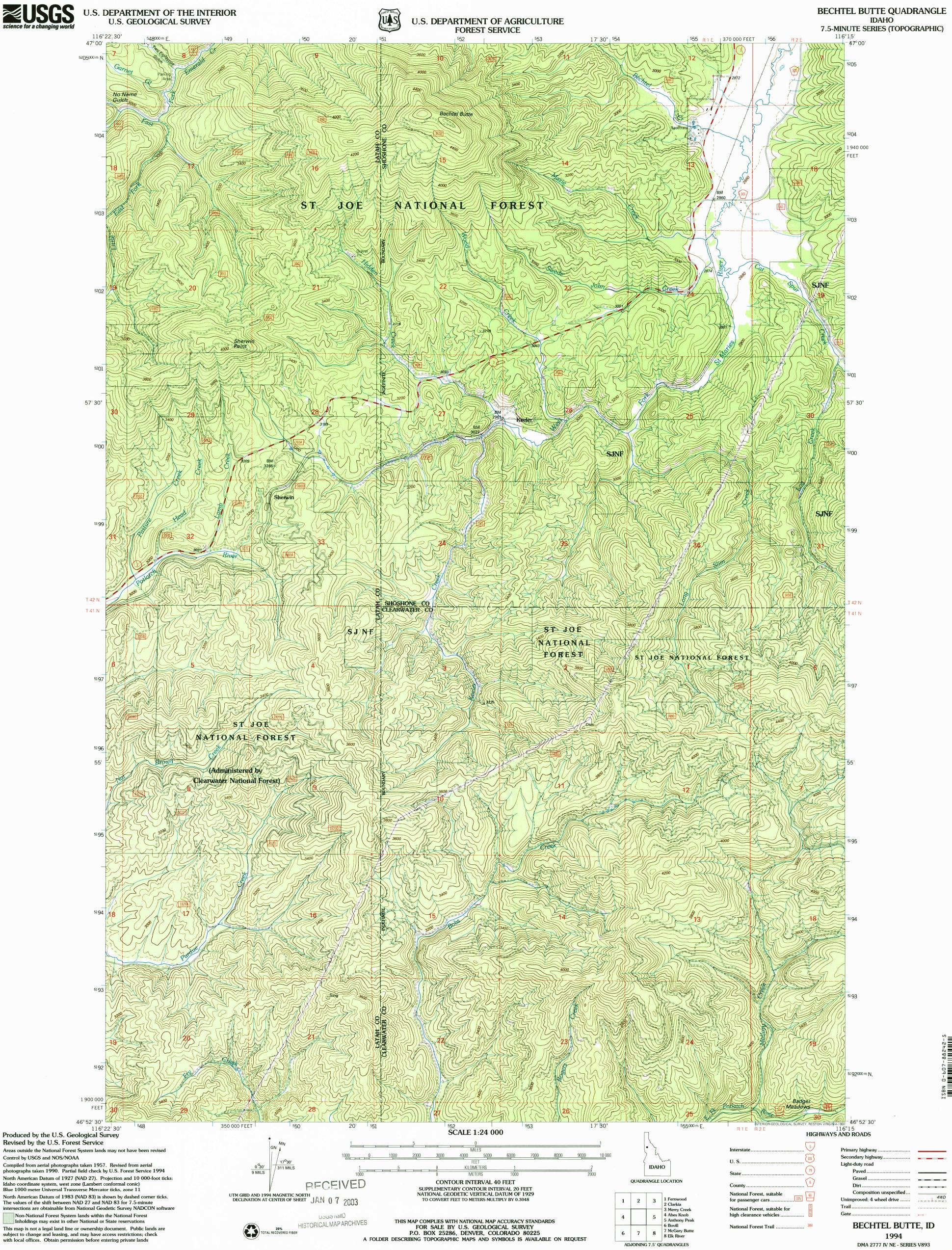
North American Datum of 1927 (NAD 27). Projection and 10 000-foot ticks: Idaho coordinate system, west zone (Lambert conformal conic) Blue 1000-meter Universal Transverse Mercator ticks, zone 11
