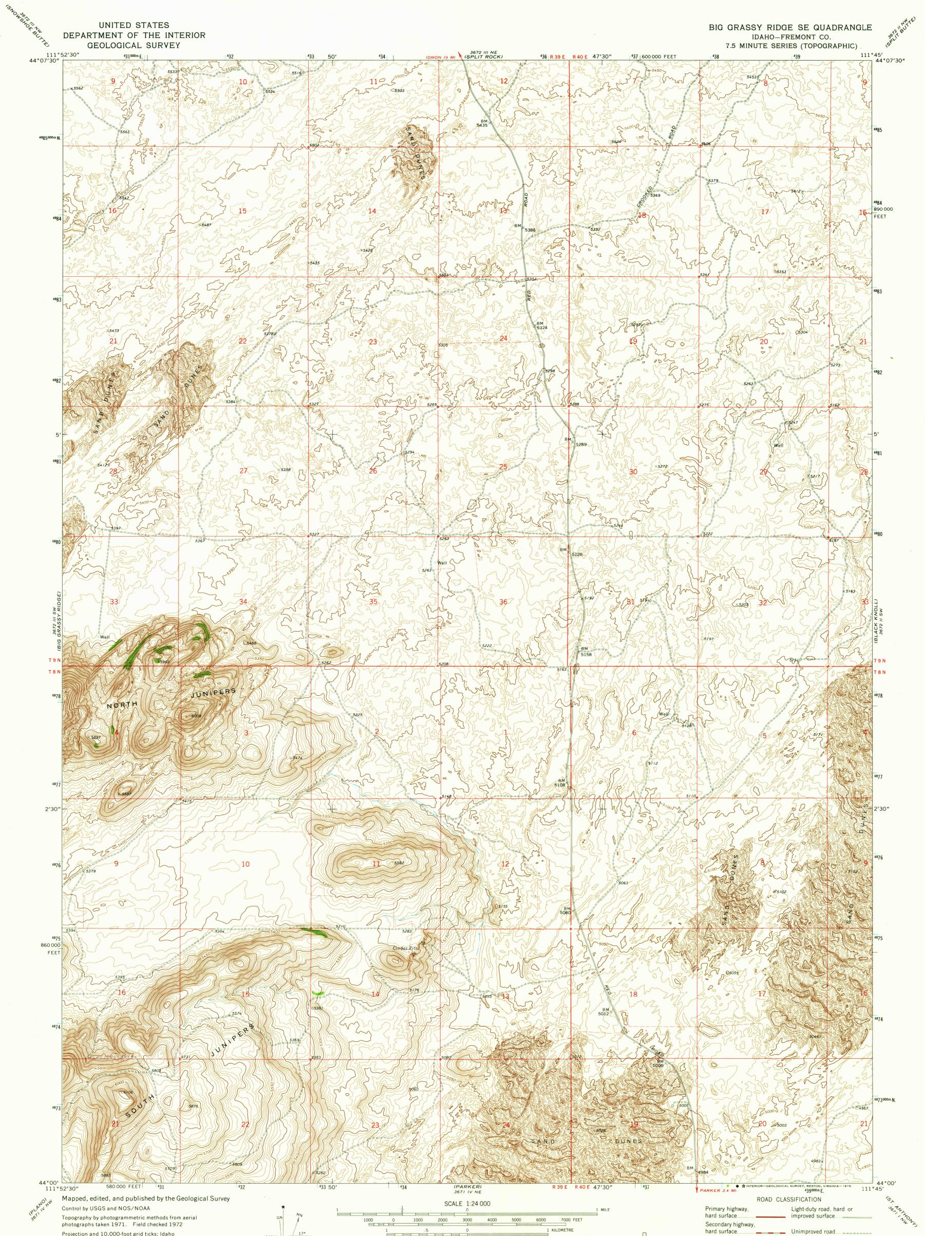
Projection and 10,000-foot grid ticks: Idaho coordinate system, east zone (transverse Mercator) 1000-metre Universal Transverse Mercator grid ticks, zone 12, shown in blue. 1927 North American datum Fine red dashed lines indicate selected fence lines
